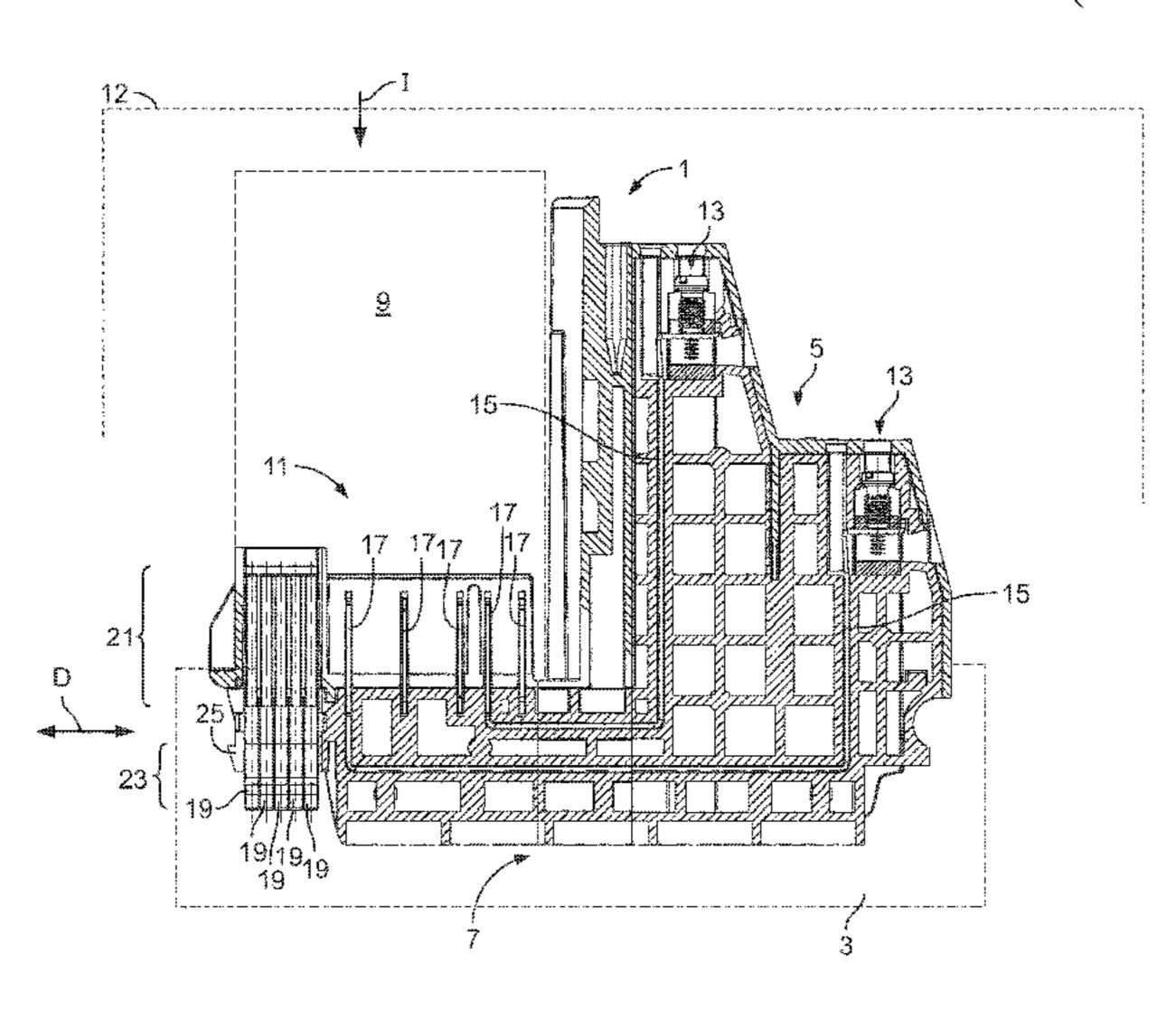
element. The movable coding element is movable from a neutral position into a coding position by insertion of a cartridge member into the cartridge receptacle. The resetting mechanism has a trigger element at least partially protruding into the module insertion path.
