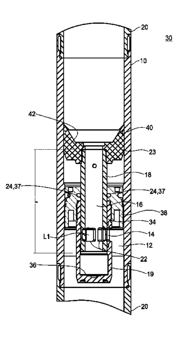
with at least one port of the sleeve. The channel element is slidable within the sleeve, upon breakage of the breakable attachment portion with a force, to move the orifice out of alignment with the port of the sleeve so that a portion of the channel element covers the port of the sleeve to block fluid flow through the port.
