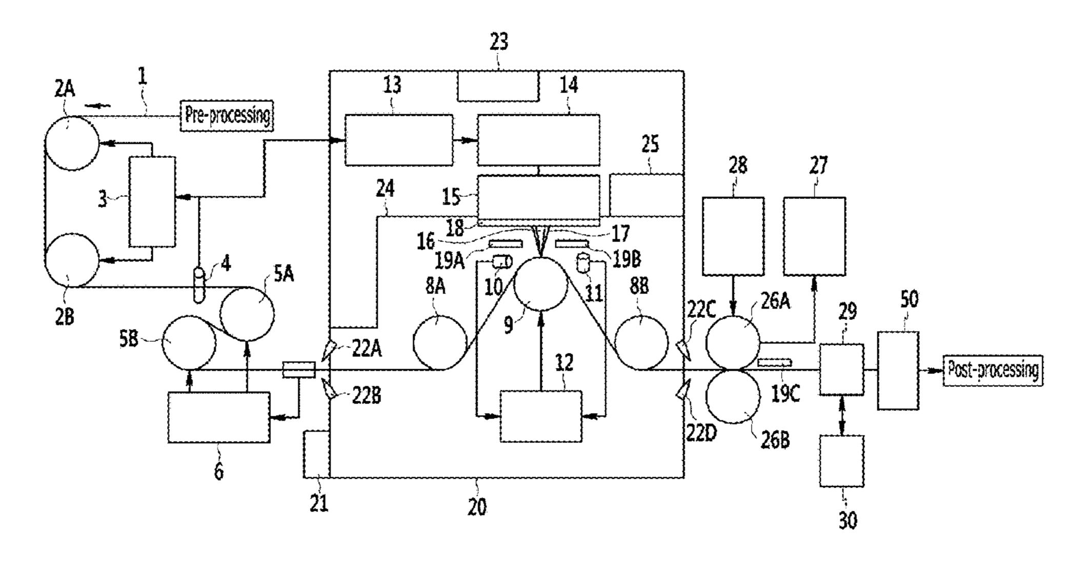
detect whether the groove is defective by confirming a machining state of a magnetic domain refined groove formed on the surface of the steel strip in a working process.
