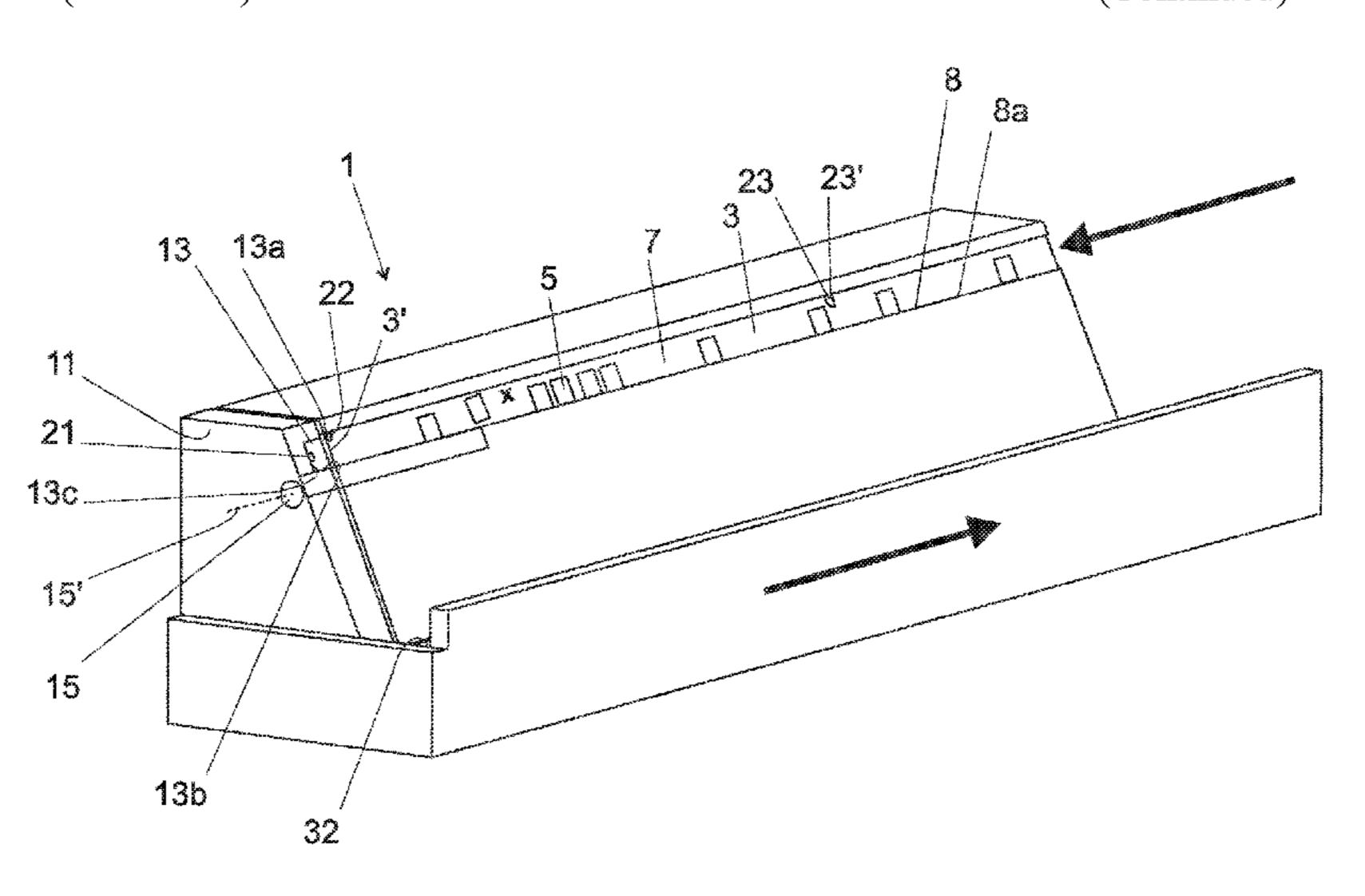
is parallel with the sloped surface of the track, so that a component can move from the track into the pocket of the pickup platform. In the second position the pocket is in a horizontal orientation.
