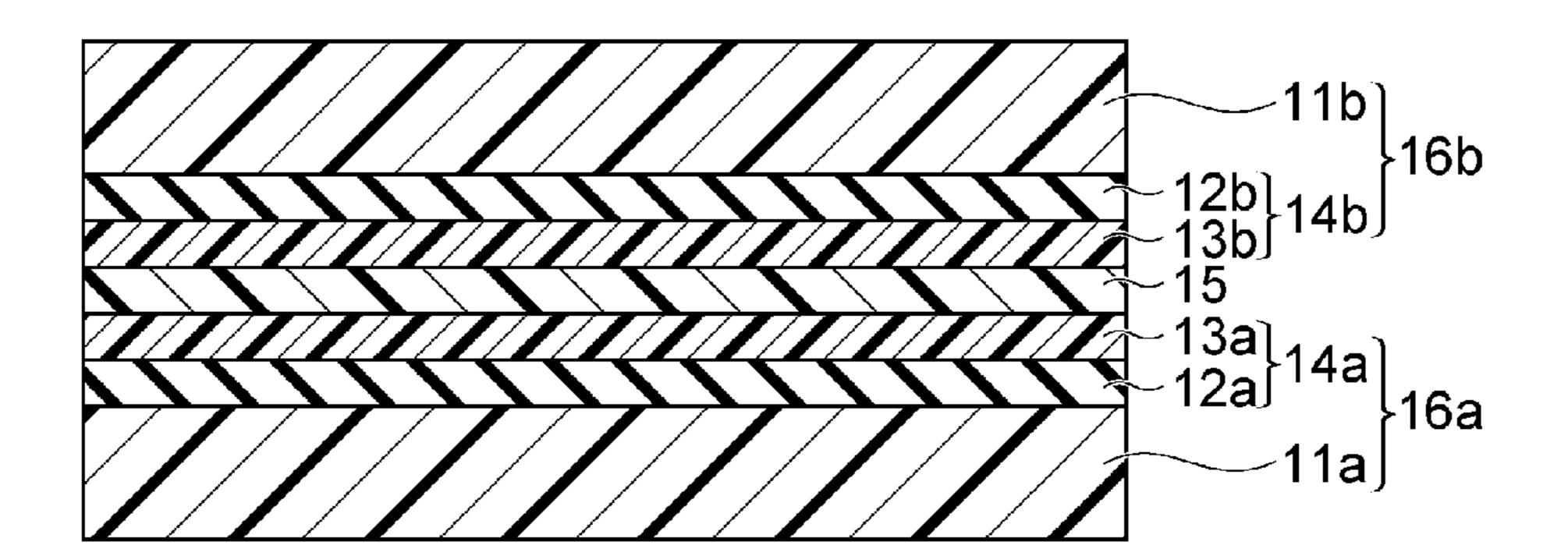
formed of an adhesive containing an epoxy resin, a curing agent having an amino group, and either a silane coupling agent having an epoxy group or a silane coupling agent having an amino group and two hydrolyzable functional groups.
