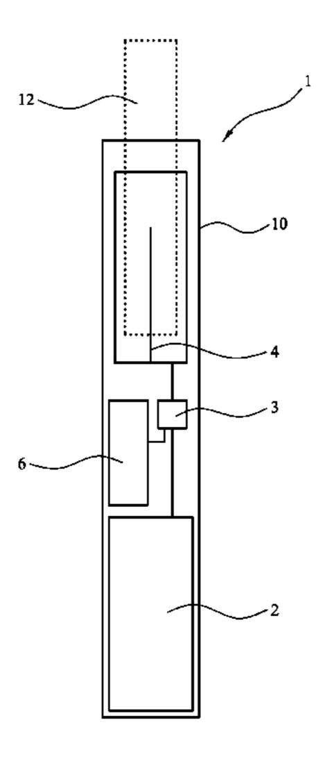
aerosol-generating element; and the method including measuring, using a measuring unit, at least one first characteristic of the battery, the at least one first characteristic comprising a temperature of the battery; and adjusting, using the control unit, a value of the duty cycle based on a predetermined rule which outputs the value of duty cycle based on the measured at least one battery characteristic. An aerosol-generating device is also provided.
