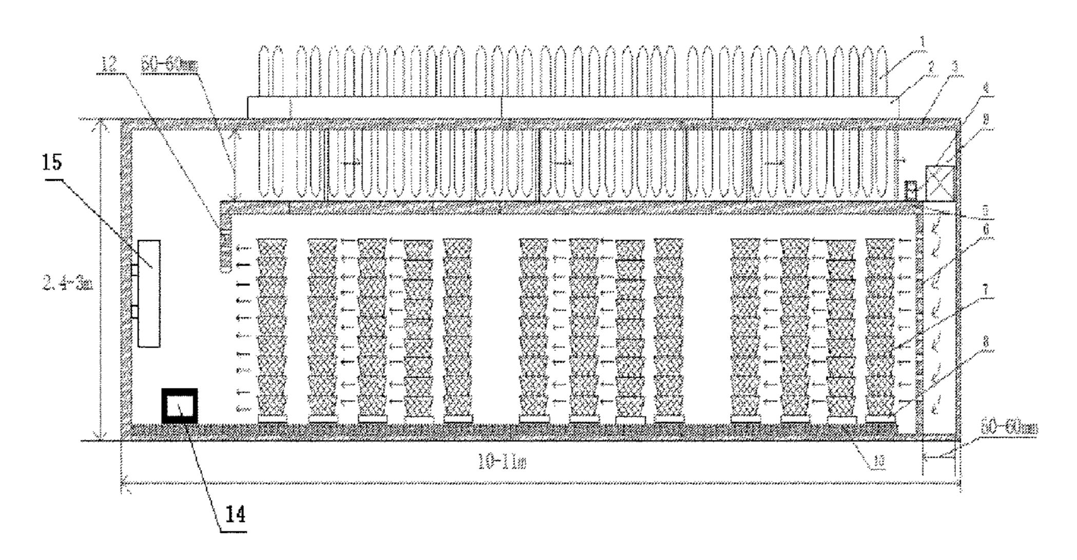
of the tunnel precooling box with a space formed therebetween; a section of wind shield is vertically and downwardly mounted to an end of the other side of the separator plate; an axial flow fan is mounted at a corner of the tunnel precooling box between the separator plate and the venting plate.
