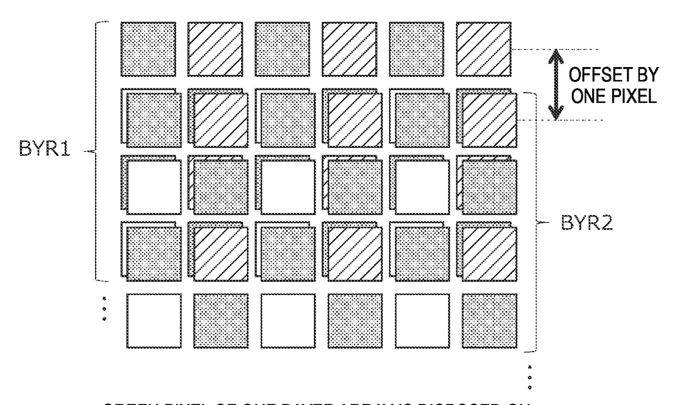
GREEN PIXEL OF ONE BAYER ARRAY IS DISPOSED ON BLUE PIXEL/RED PIXEL OF THE OTHER BAYER ARRAY
