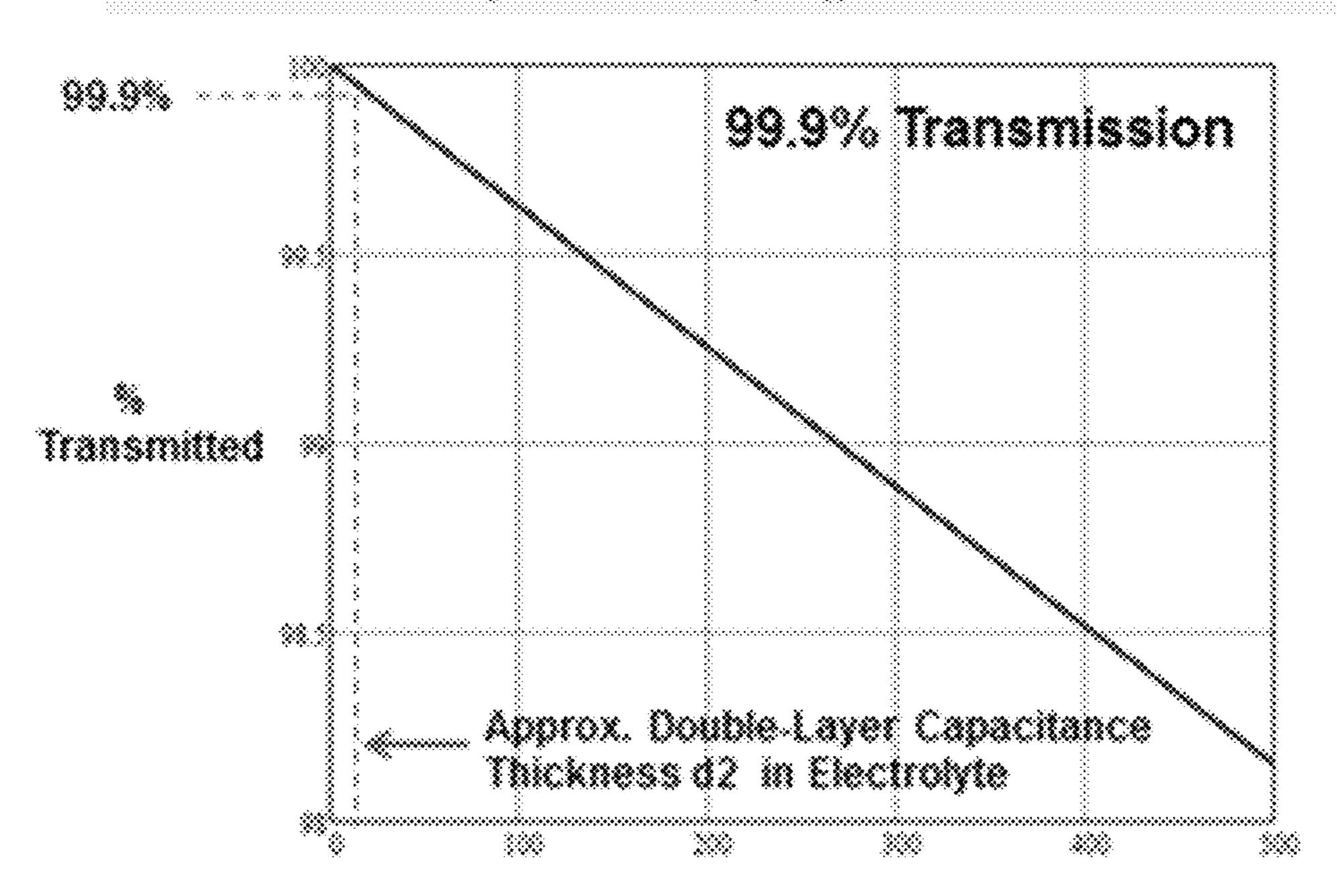
Double-Layer Capacitance thickness d2 (Angstroms)
