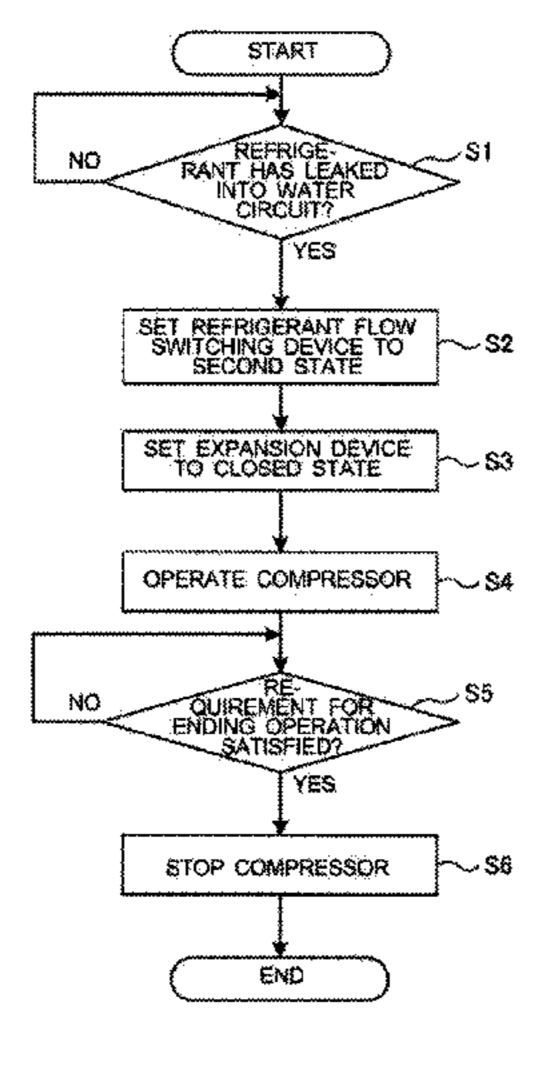
heat exchanger and one of the branching part and the joining part, or at the load-side heat exchanger. When leakage of refrigerant is detected, the state of a refrigerant flow switching device is set to a second state, an expansion device is set to a closed state, and a compressor is operated.
