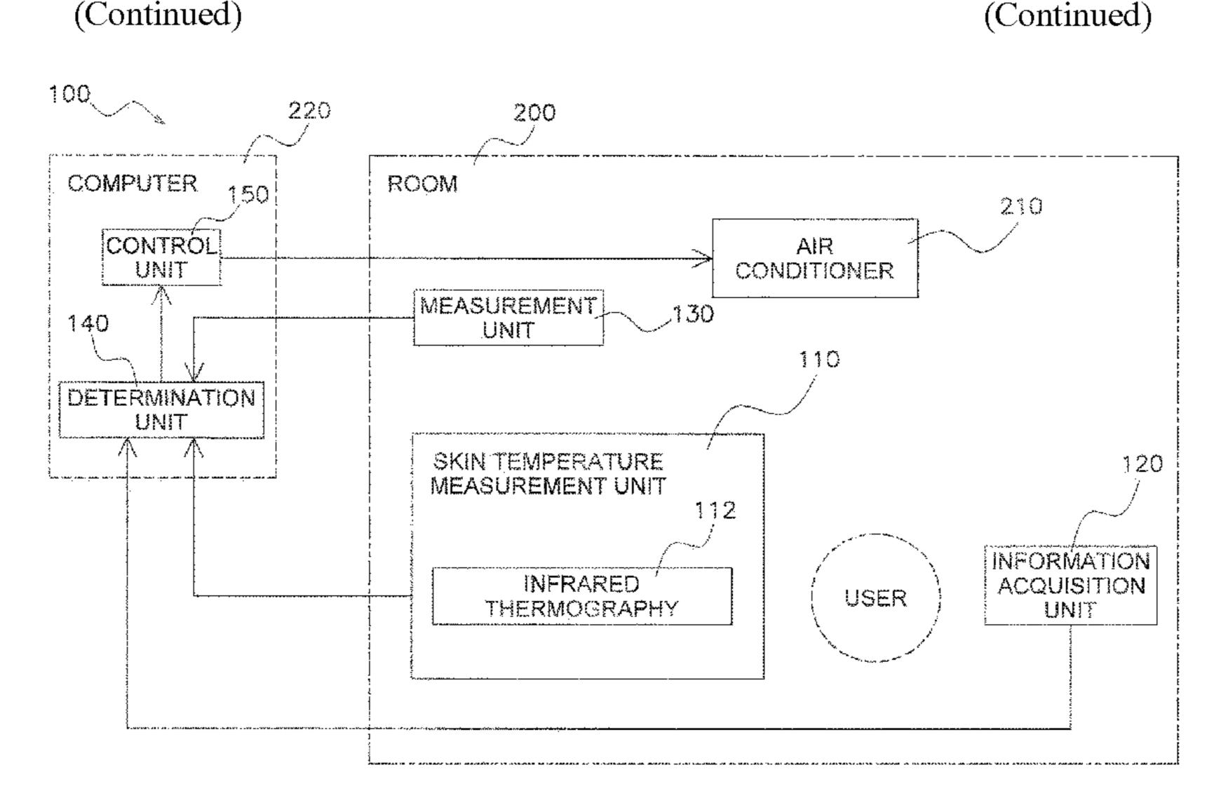
information acquisition unit acquires thermal sensation information of the user regarding the space where the user is present. The determination unit determines a comfortable skin temperature range in which the user feels comfortable, based on a skin temperature of the user obtained at the time of acquiring of the thermal sensation information. The control unit controls the air conditioner based on the comfortable skin temperature range determined by the determination unit.
