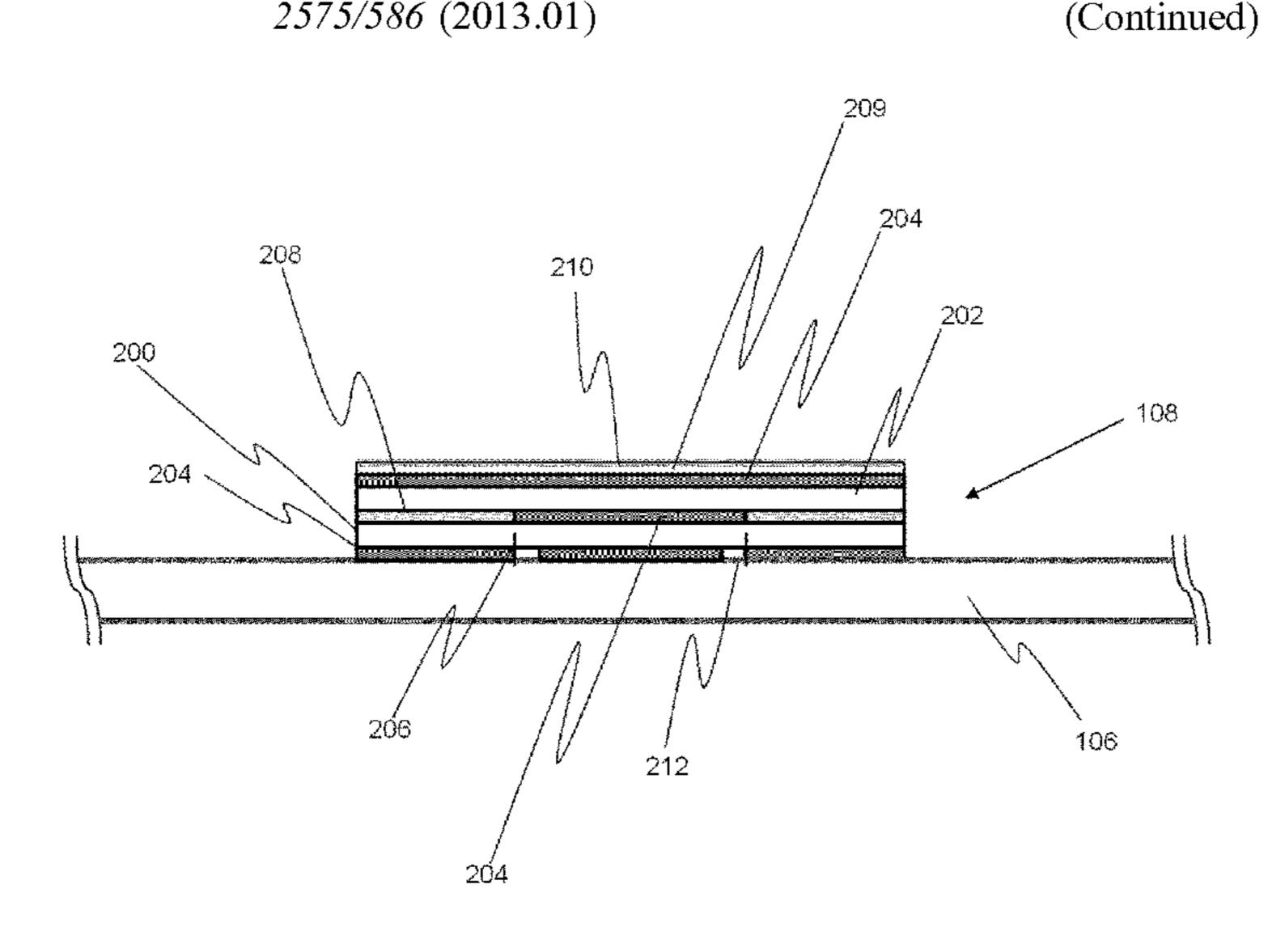
lower periphery of the cut-out of the first layer. The second adhesive is a removable adhesive and a peel strength for peeling the first layer from the package is greater than a peel strength for peeling the second layer from the first layer. The second layer of the self-adhesive reclosable sticker is permanently affixed to the inner surface of the lid.
