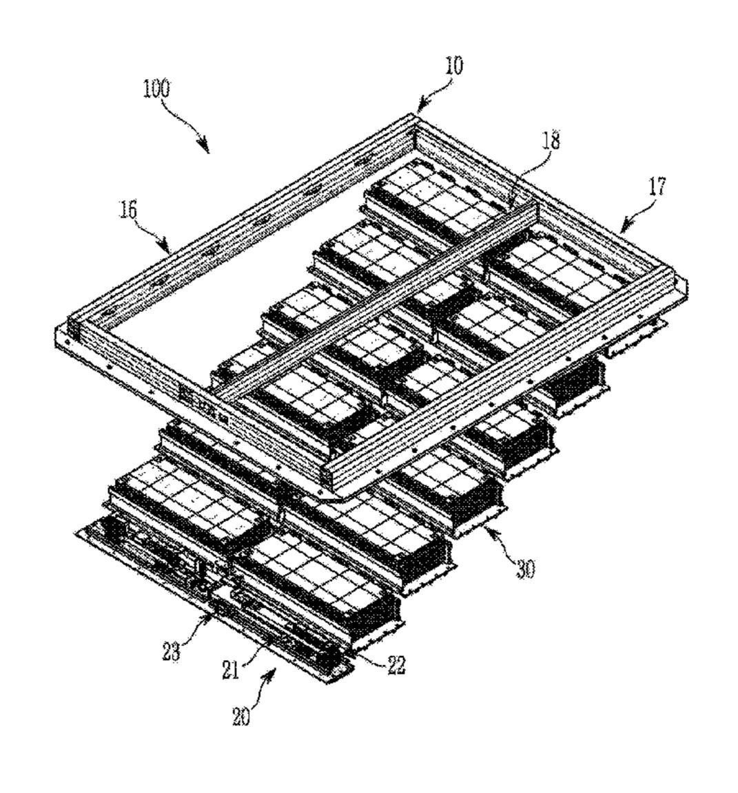
corners of the bottom plate, a pair of end plates perpendicular to the bottom plate and the side wall, extending along two facing corners of the bottom plate, and mechanically connected to the side walls and/or the bottom plate to fix the plurality of battery cells together. A cell cover extends parallel to the bottom plate to form a receiving space of the battery submodule along with the bottom plate, the side wall, and the end plate.
