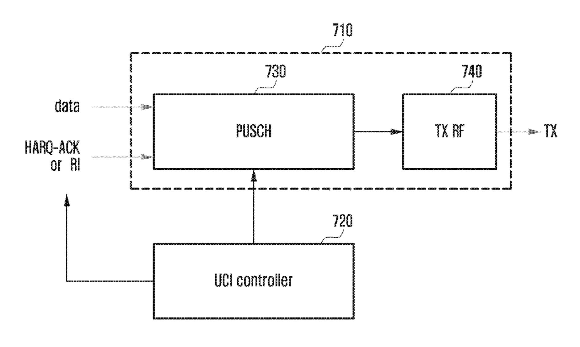
(ACK)/negative ACK (HACK) information corresponding to downlink data received from a corresponding base station is provided.
