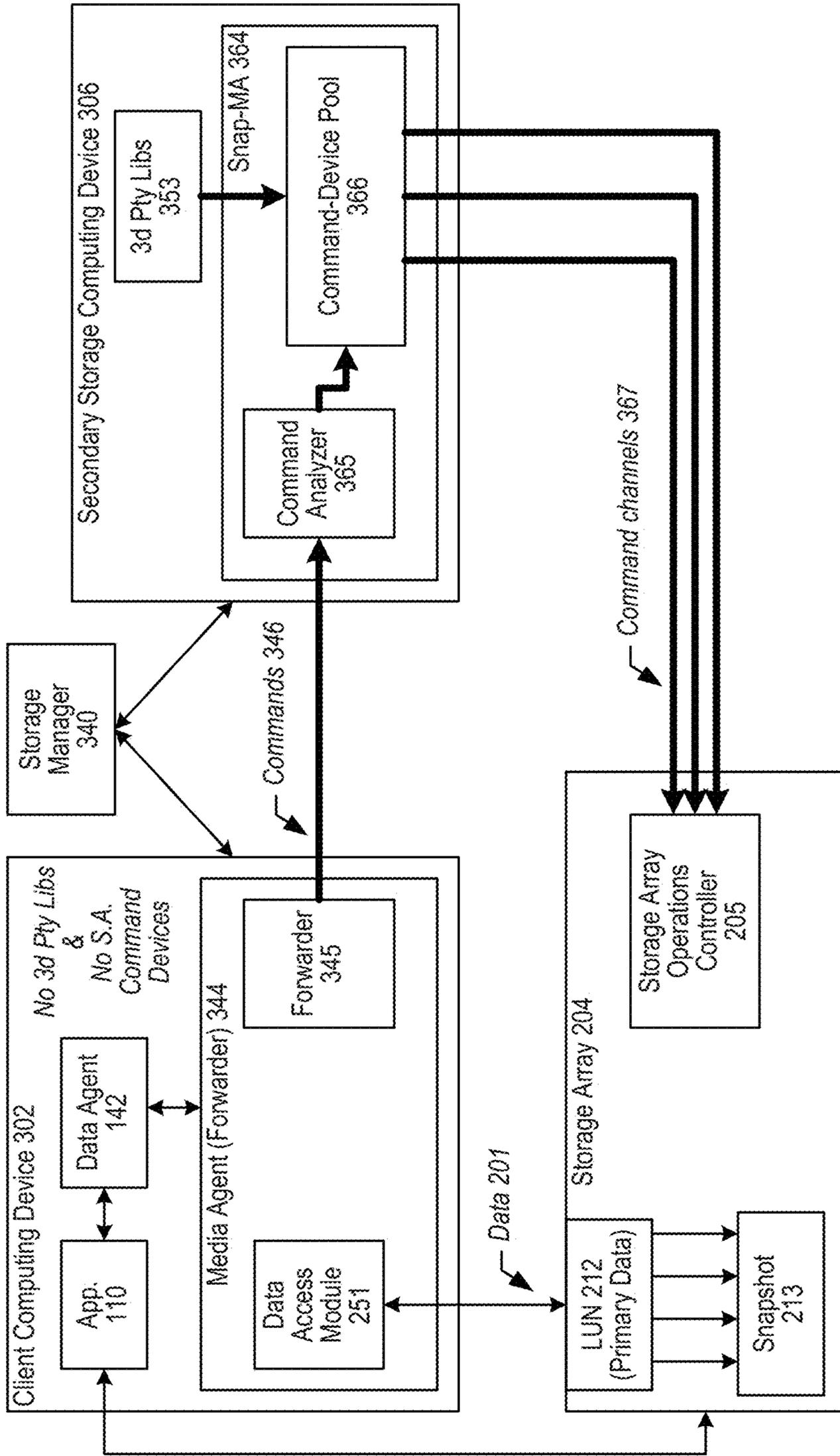
**FIG. 3B** System 300 Detail Of A Forwarder Media Agent On A Client Computing Device And A Snap-MA
