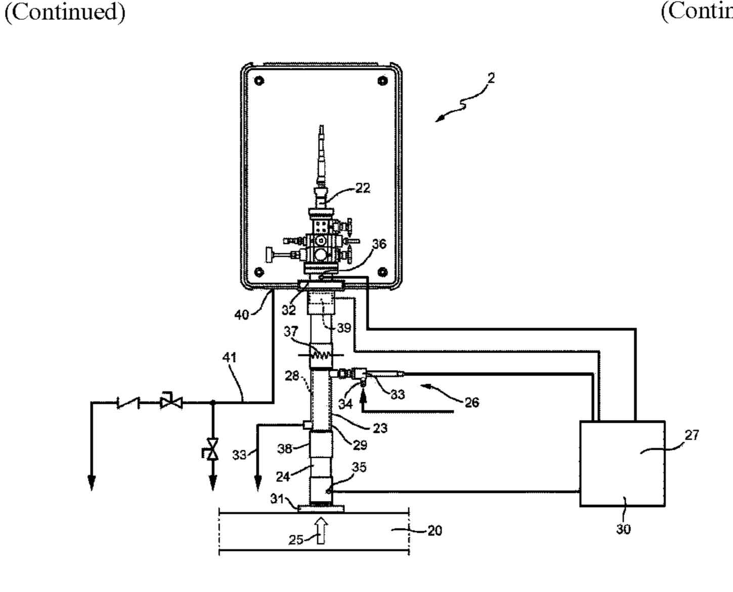
portion of the conduit configured to adjust the temperature of the sample stream circulating in the conduit.
