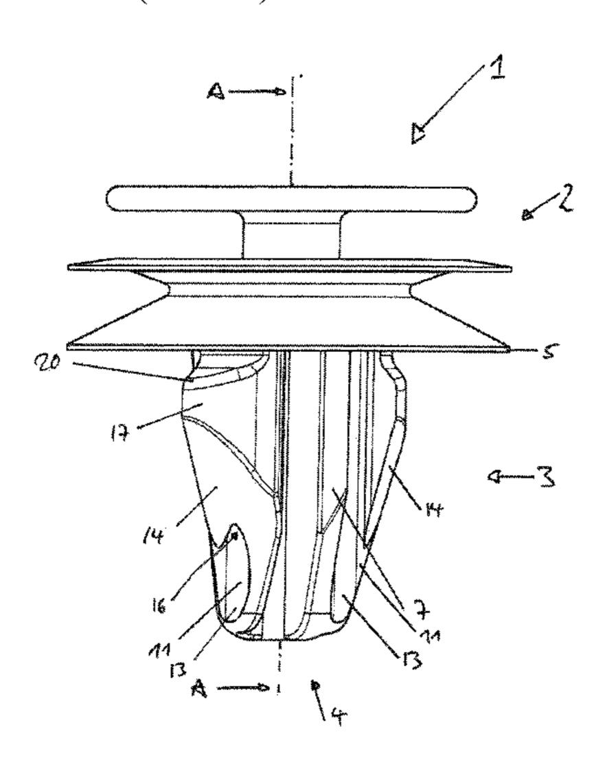
other end to the second section, the second section extending in a different direction from the first section, the first section is connected directly to the head.
