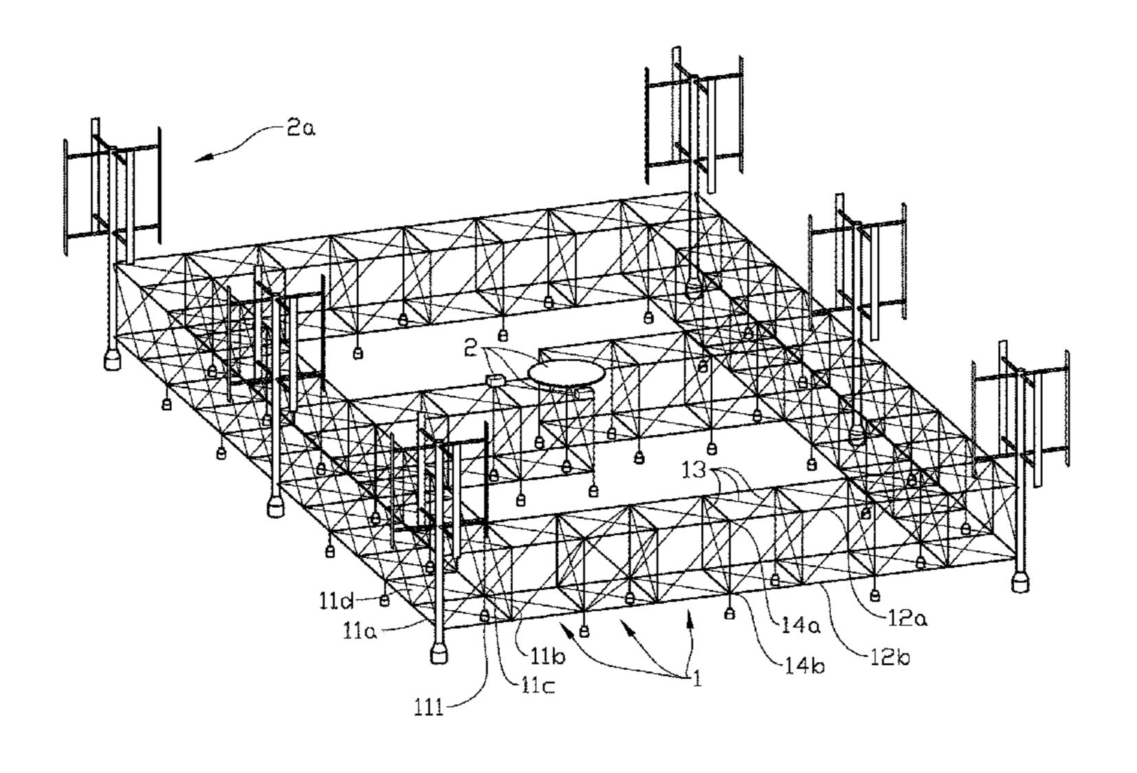
plane and in the same frame module being connected by elastic tensile elements. Some columns form containers with submersible portions with positive buoyancy, and adjacent frame modules sharing at least one column.
