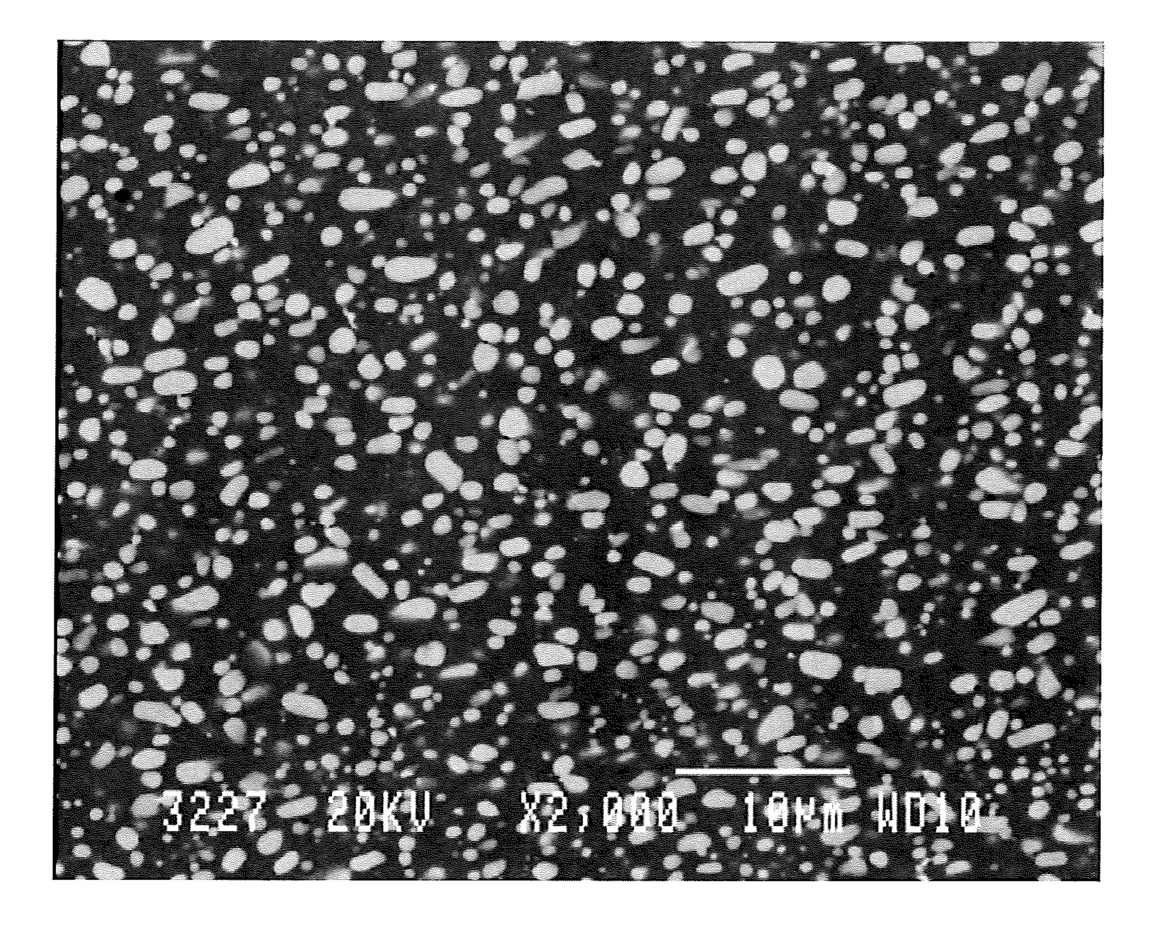
Microstructure of the inventive alloy. The white phase is  $Mo_2FeB_2$ . The length of the bar is  $10~\mu m$ .
