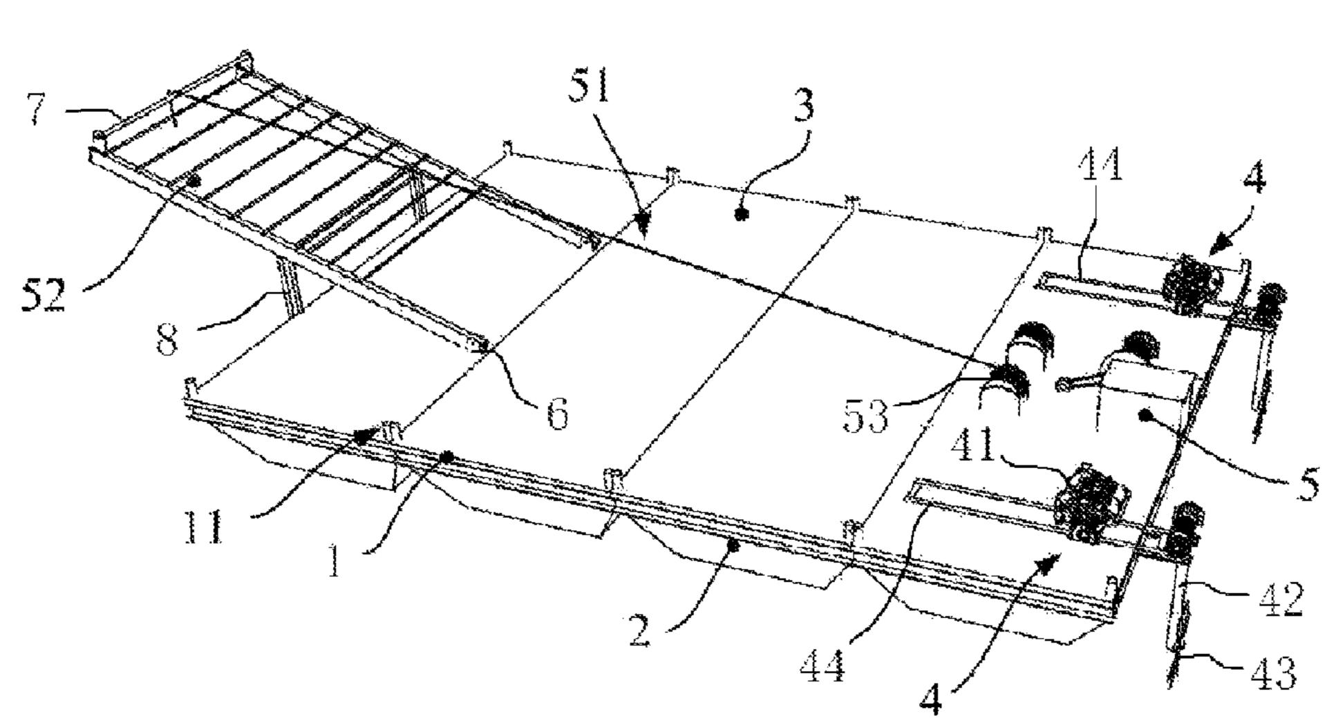
platforms collectively form a deck. A transportation method transports goods to the platform by means of a hoist, and a hoist bracket with a rotating roller. The platform can achieve standardized production, and is flexible and has multiple functions.
