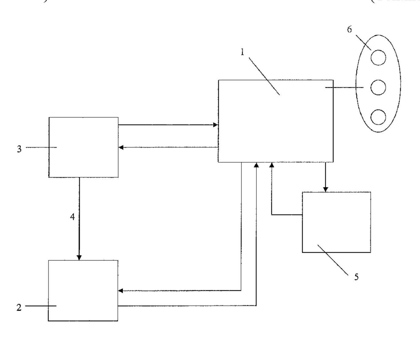
said second pressure measuring device being connected to the computing device. A feedback indicator is connected to the computing device and is adapted to indicate the viability of the tissue calculated by the computing device on the basis of the measured local and systemic perfusion pressures. The invention also includes a method of predicting the viability of the body tissue and to the first pressure measuring device.
