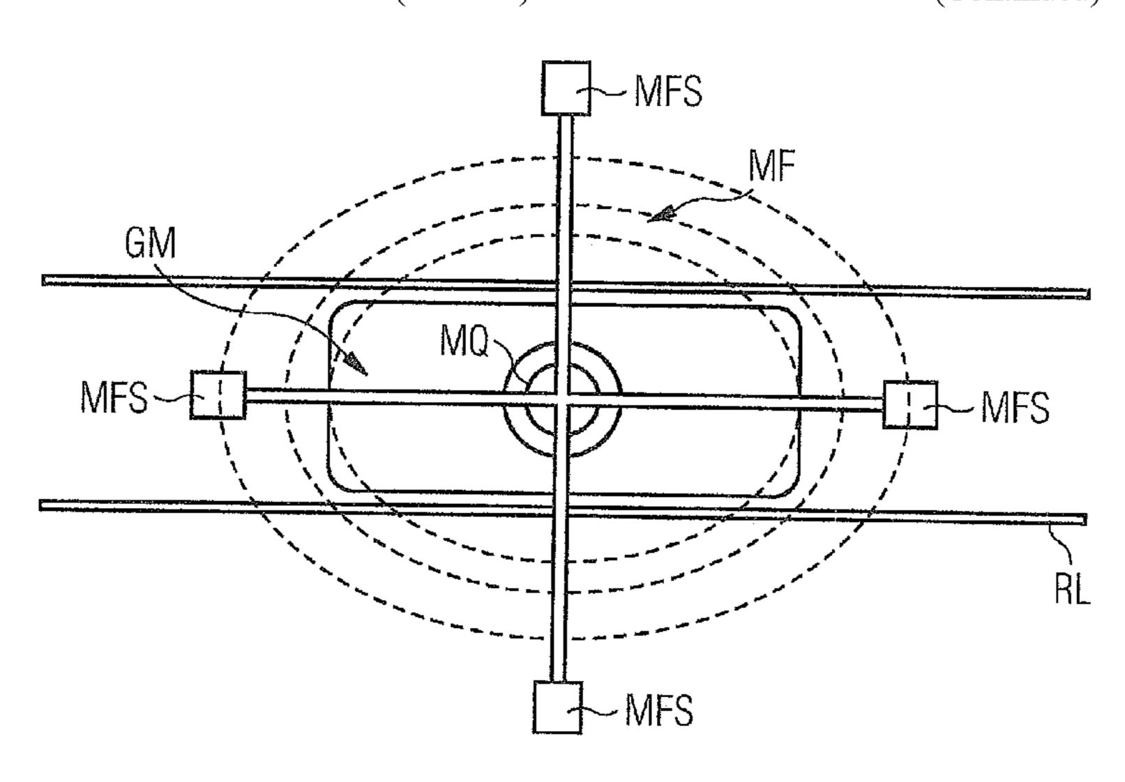
positioning the unmanned aerial vehicle at a defined distance from the at least one geopig, and a device is provided for determining the location of the at least one geopig from the position of the unmanned aerial vehicle and the defined distance between the at least one geopig and the unmanned aerial vehicle.
