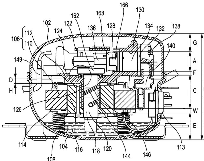
(122), and a thrust bearing that supports a load of shaft (118) in a vertical direction. The thrust bearing includes an upper race in contact with a flange portion of shaft (118), a lower race in contact with a thrust surface of cylinder block (124), and a rolling element. An overall height of sealed container (102) is sized not to exceed a length six times larger than a diameter of piston (128).
