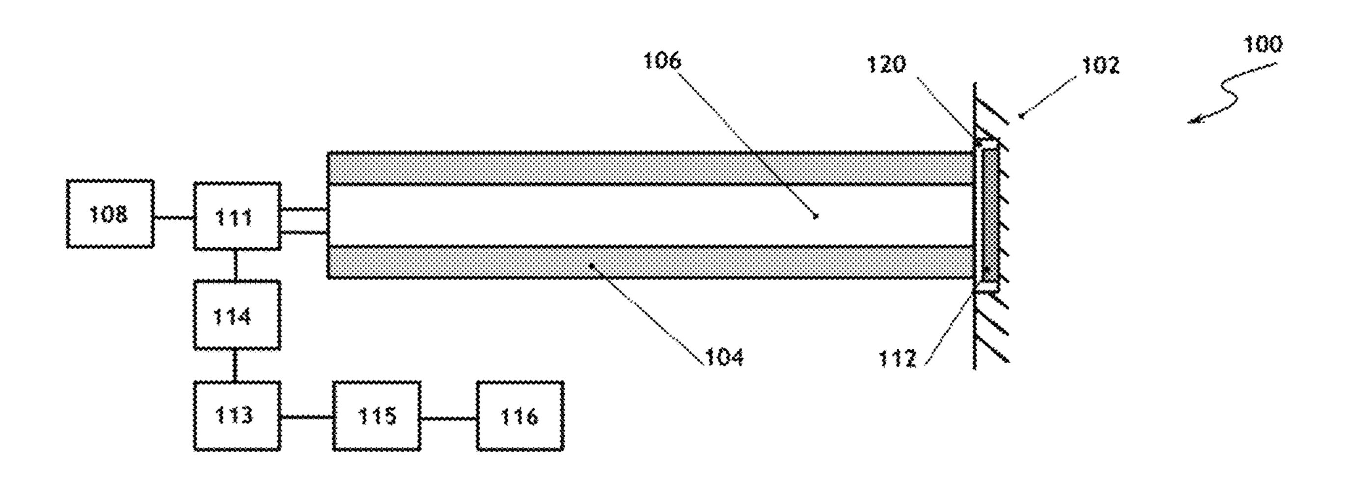
time of the phosphor luminescence is a function of the measuring parameter.
