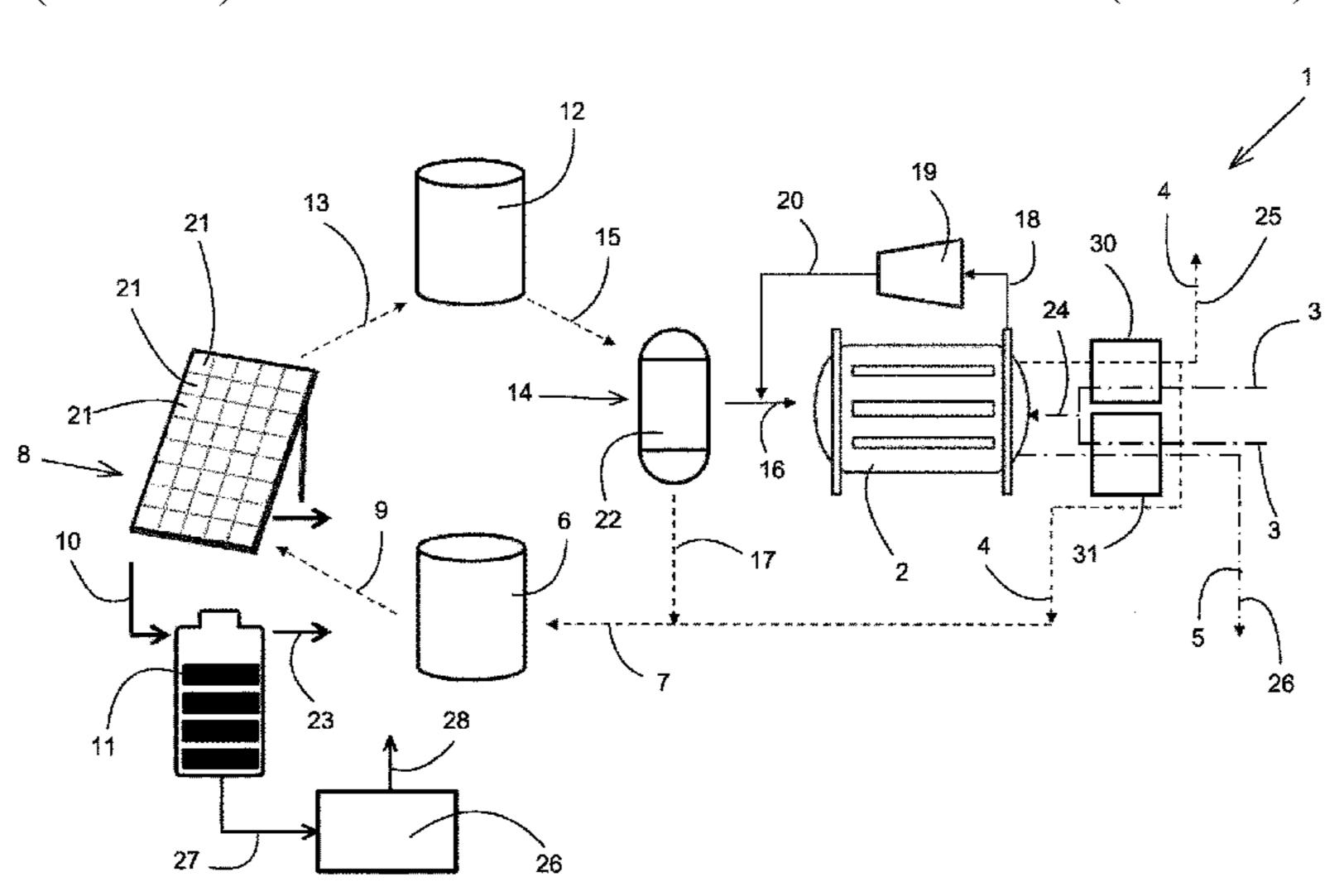
lation (MED) combined with vapour compression (VC) being able to work 24 hours a day only on solar energy.
