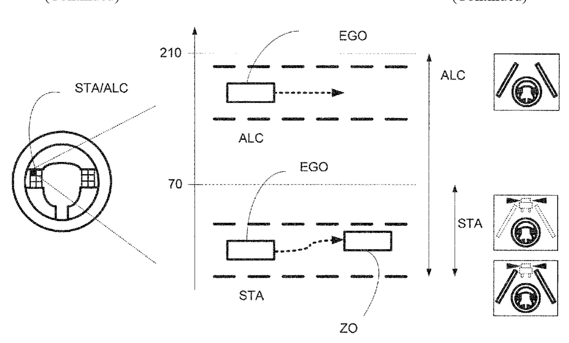
activated and deactivated by a single on-/off-button. The driver assistance system is characterized by a special combination of the sub-functions track guiding assistance and traffic jam assistance. They each take turns depending on the presence of conditions, which are defined differently for each sub-function.
