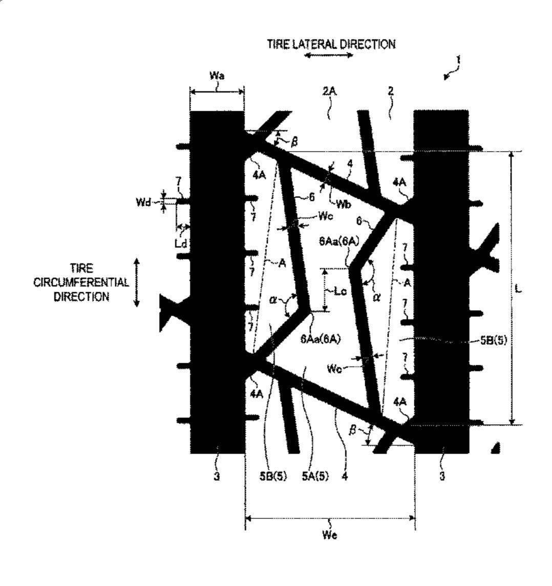
being disposed inward in the lateral direction, and bend points of the bent portions being disposed at positions offset from one another in the circumferential direction.
