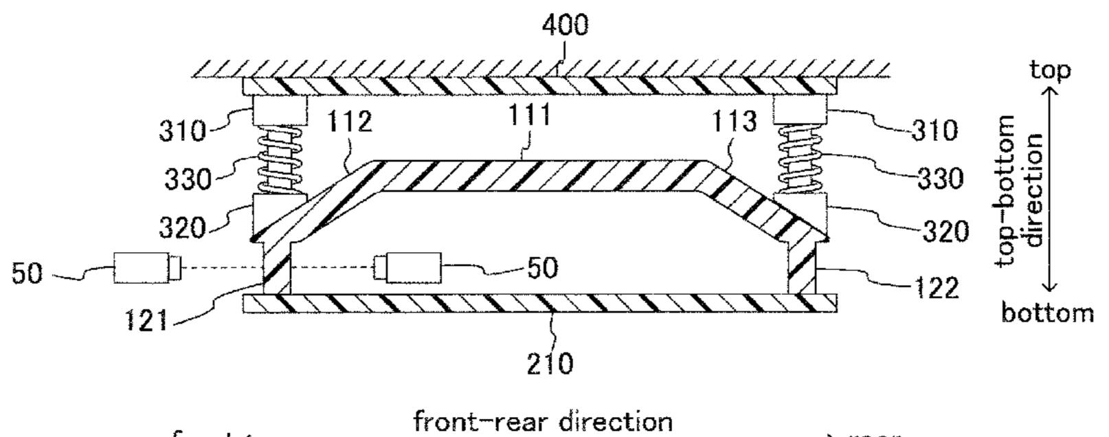
front ← → rear melted portions, whereby the first member and the second member are welded together.
