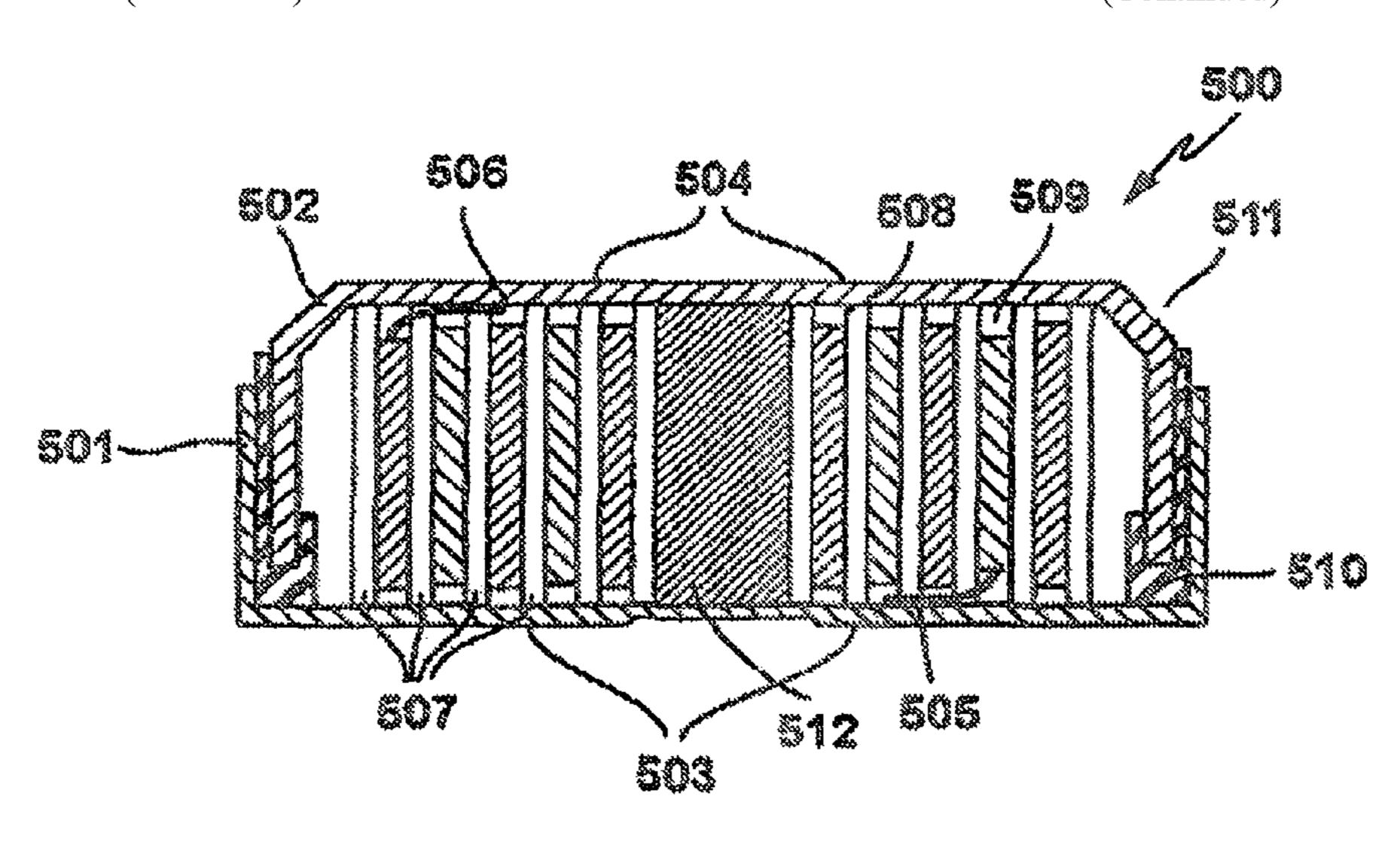
first output conductor. An insulator is disposed between an end face of the electrode-separator assembly winding and the first output conductor, wherein the first output conductor is welded to the first of the flat bottom area or the flat top area.
