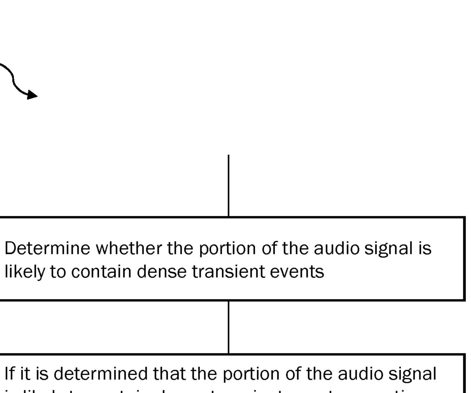
If it is determined that the portion of the audio signal is likely to contain dense transient events, quantize the portion of the audio signal using a quantization mode that applies a substantially constant signal-tonoise ratio over frequency for the portion of the audio signal
