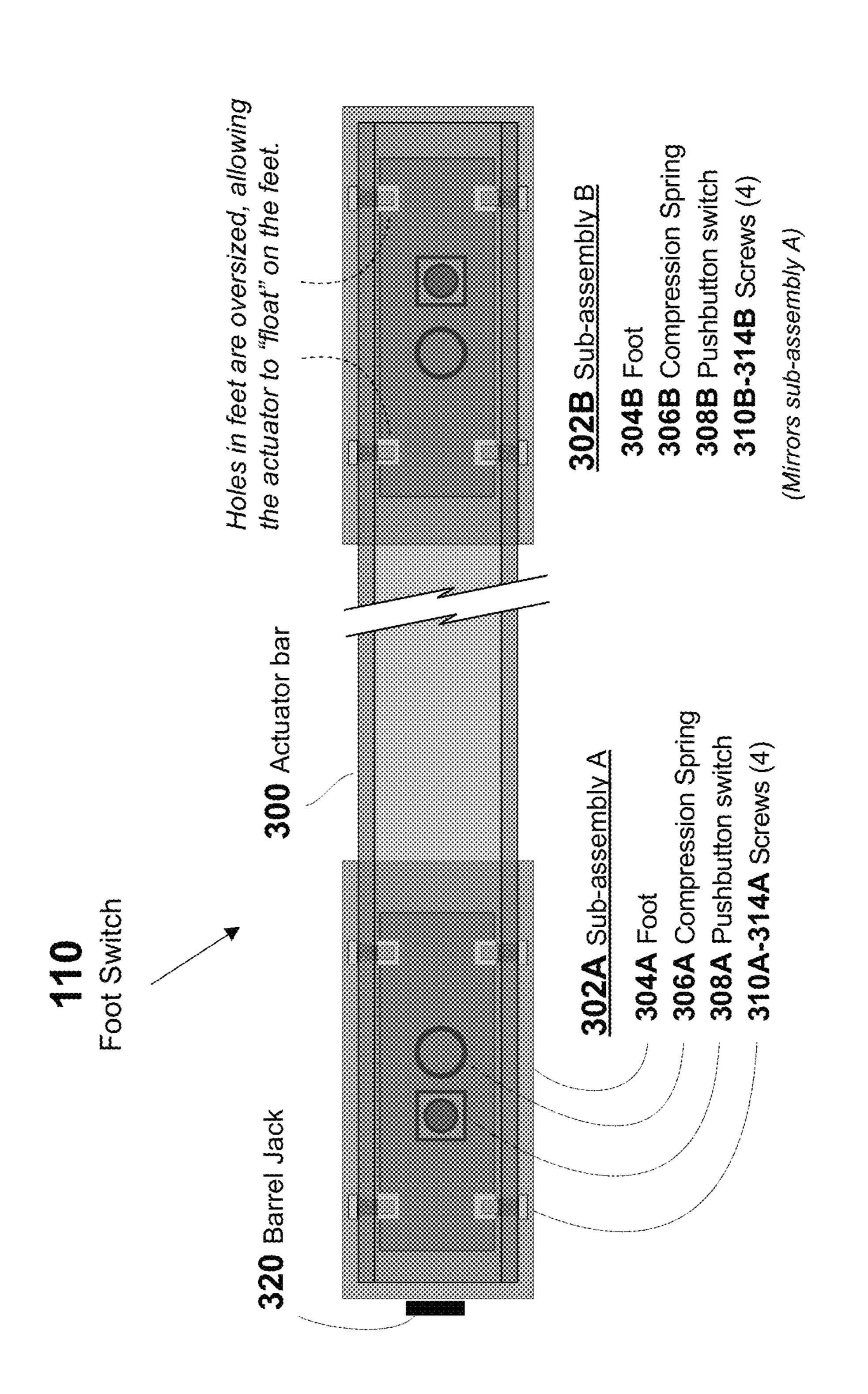
FIG. 3C - Foot Switch Top View
