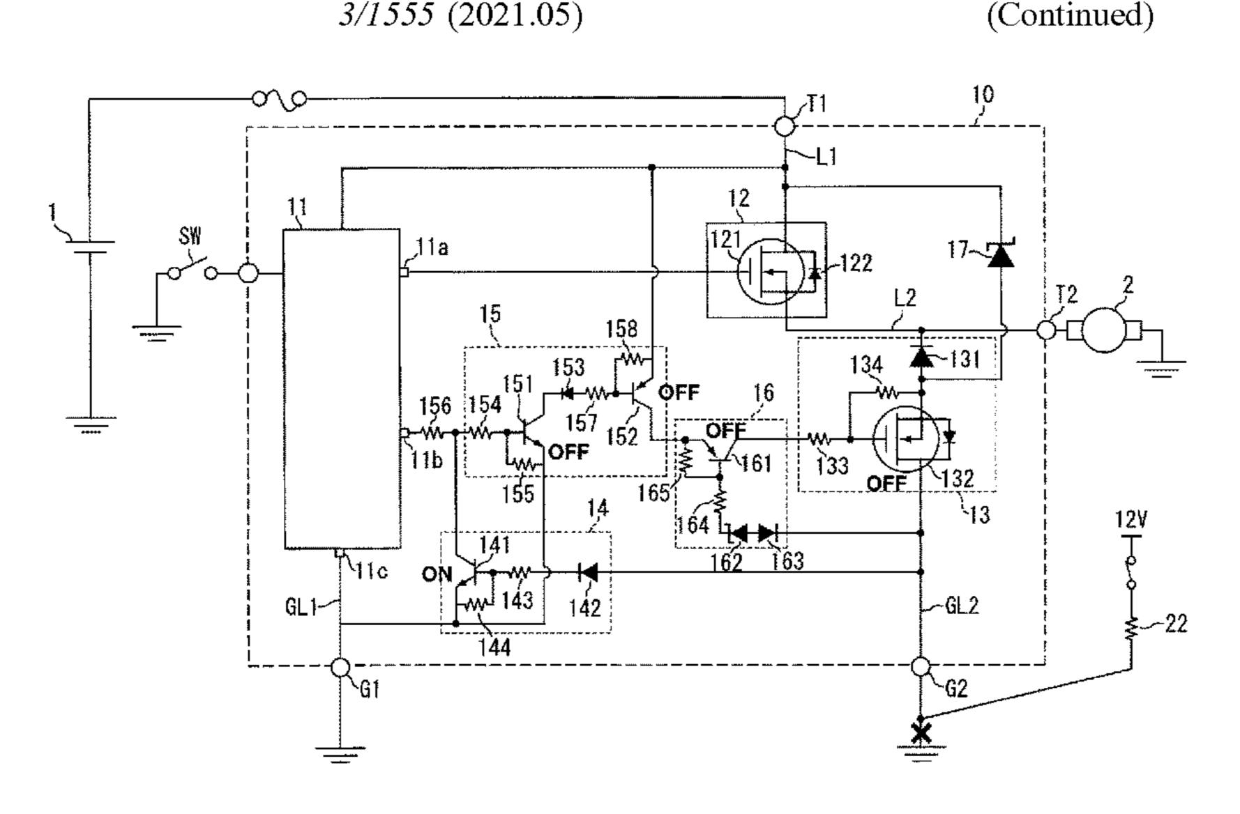
terminal to the first terminal when a rise in a potential difference between the first terminal and the second terminal is detected.
