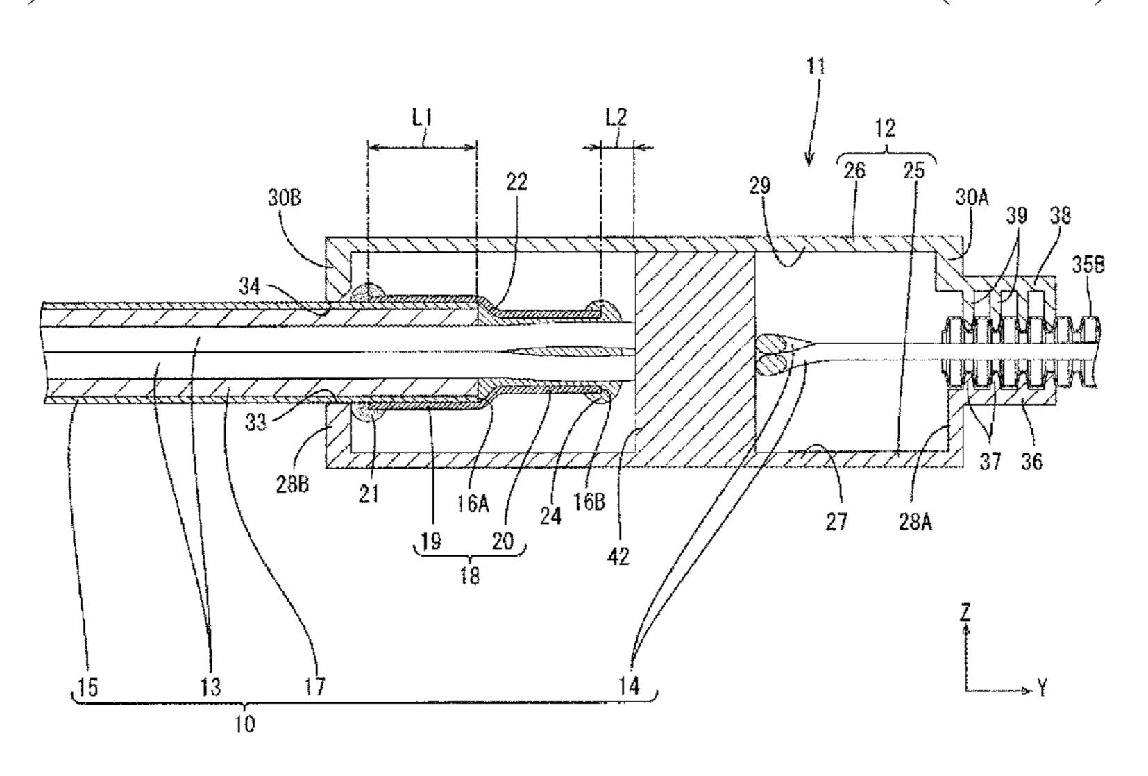
covering portion and the power line and the signal line to prevent water from entering the gap between the electric wire covering portion and the power line and the signal line; and a protector that holds the heat-shrinkable tube therein and has a stopper located near a front end of the heatshrinkable tube.
