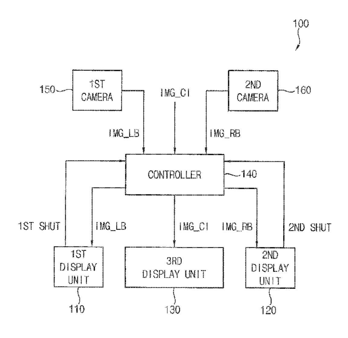
display unit in response to the second shut-down control signal.
