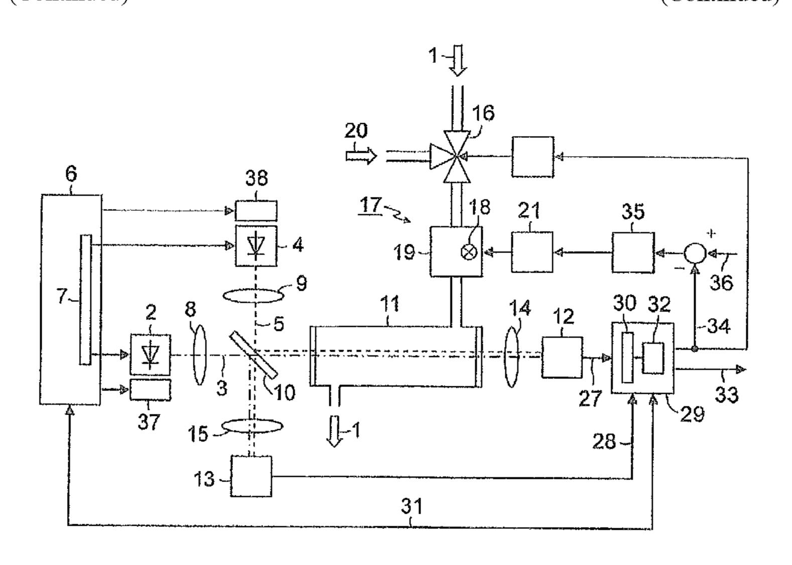
continuous measurement of nitrogen oxides in exhaust gases with a low outlay on equipment.
