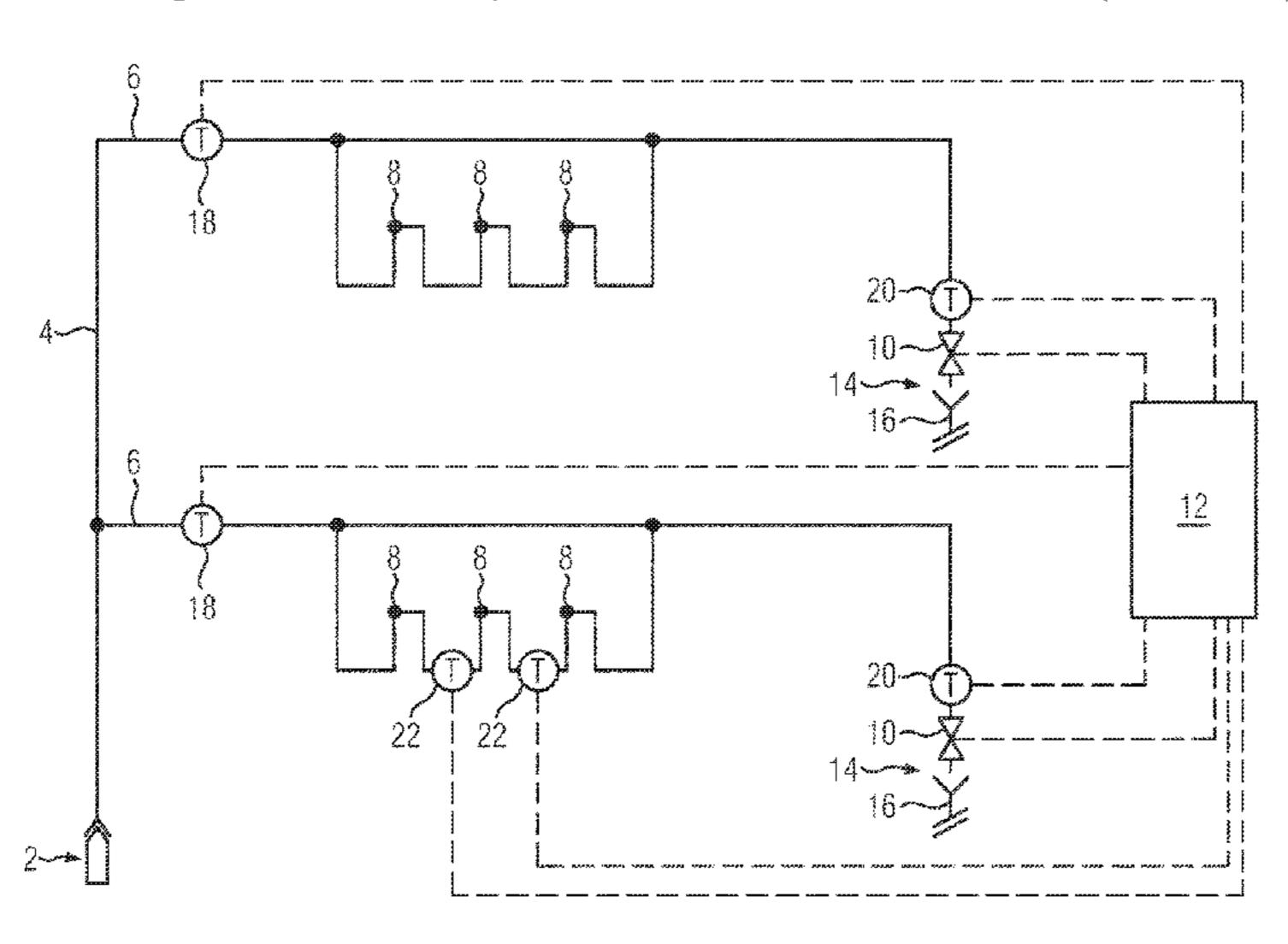
be suspended or postponed on the basis of a temperature difference between a measured value of the first temperature sensor (18) and a measured value of the second temperature sensor (20). In a secondary aspect, the present invention provides a method for flushing such a system.
