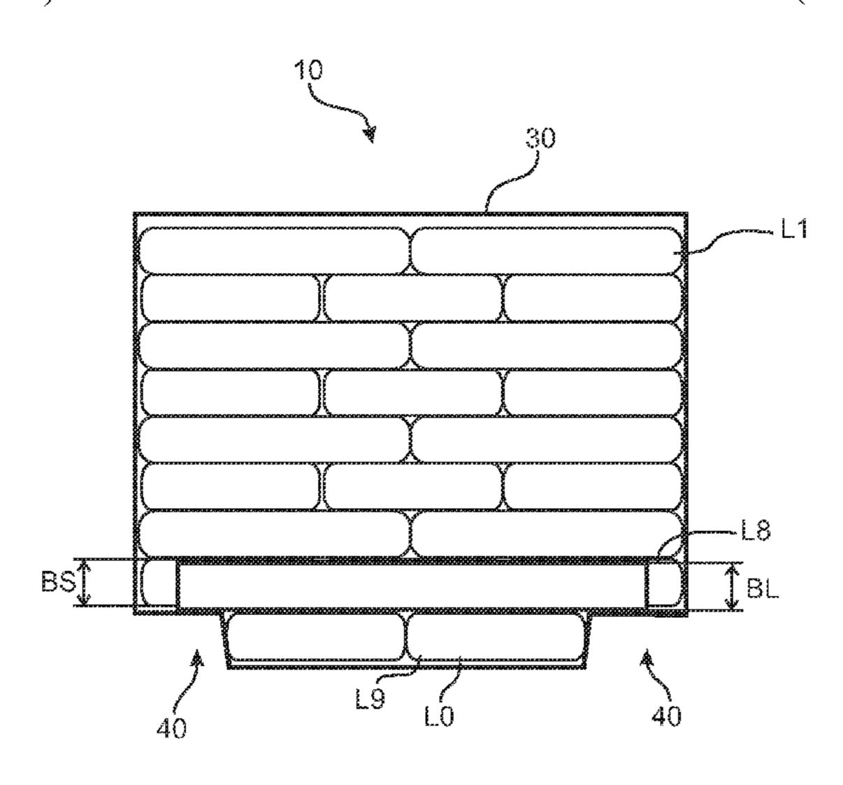
extends along the lateral side (22) of the sacks (20) of one of both neighboring layers (L8, L9) and transverse to the elevating recesses (40).
