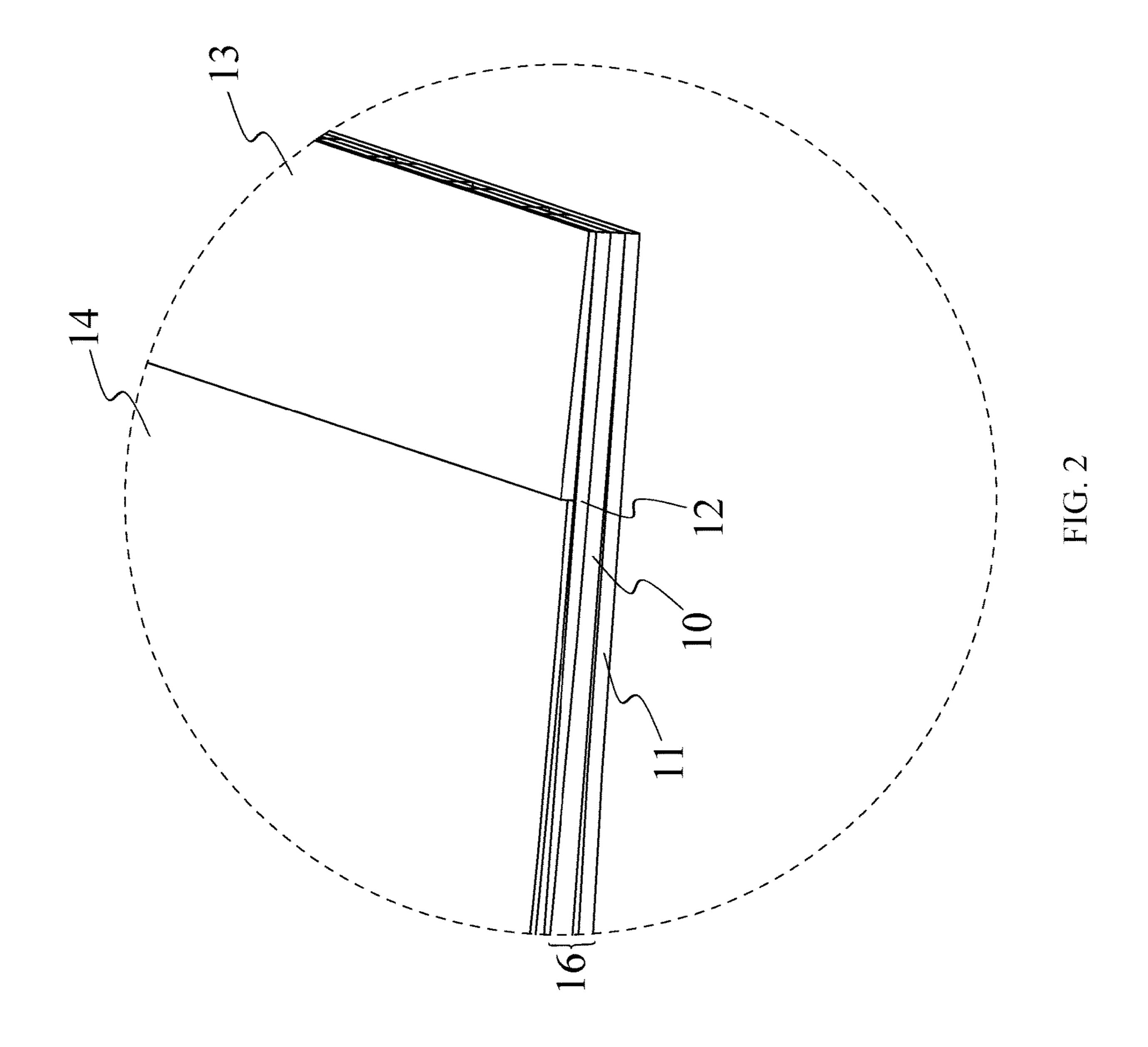
(A) Providing at least one scrim, a film exudate, a quantity of primary adhesive, at least one susceptor, a quantity of flocking material, wherein the scrim, the film exudate, and the quantity of flocking material are made of a thermoplastic material
