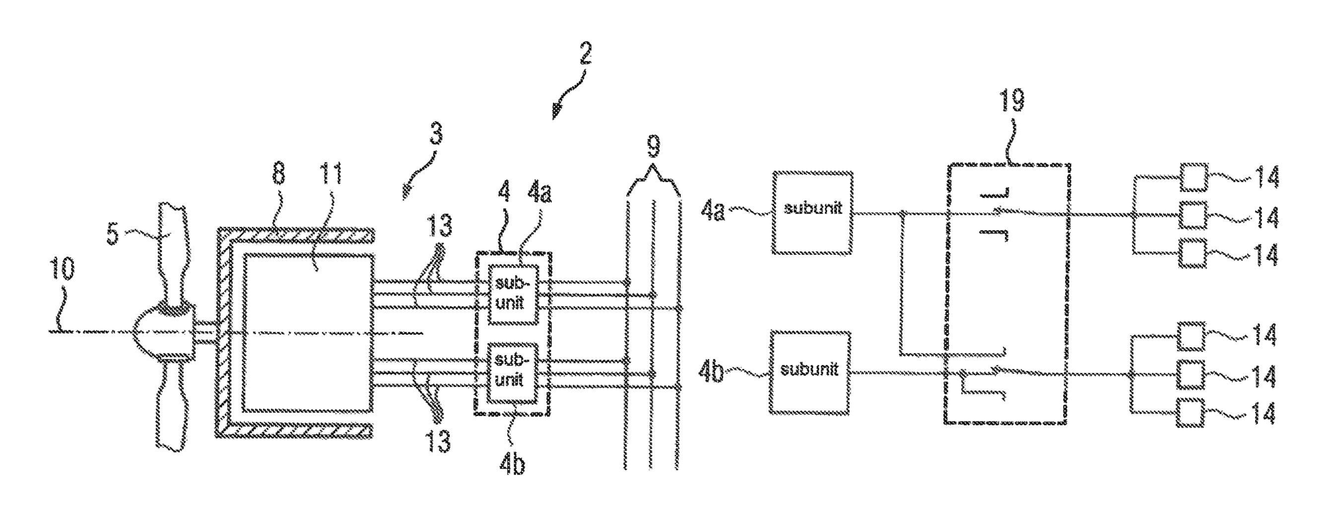
segments when viewed about the rotation axis. The terminals of the stator segments are connected to the same sub-unit within each group, but connected to different sub-units from group to group of stator segments.
