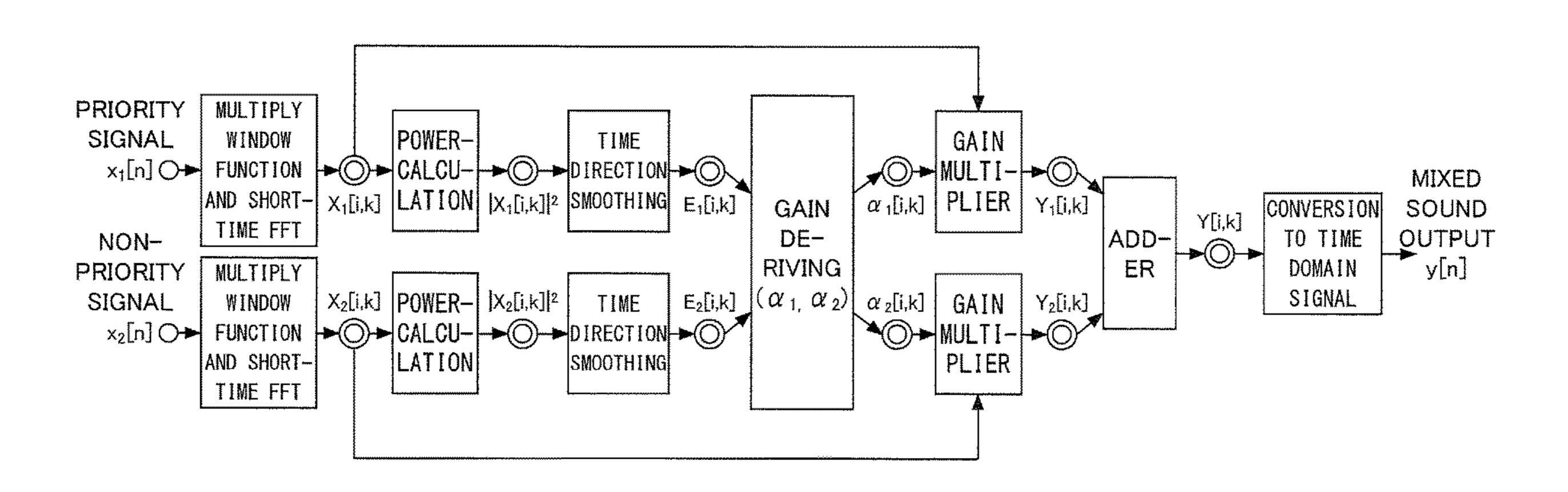
so that predetermined conditions for simultaneous gain generation are satisfied at least at the first channel and the second channel among the first channel, the second channel, and the third channel.
