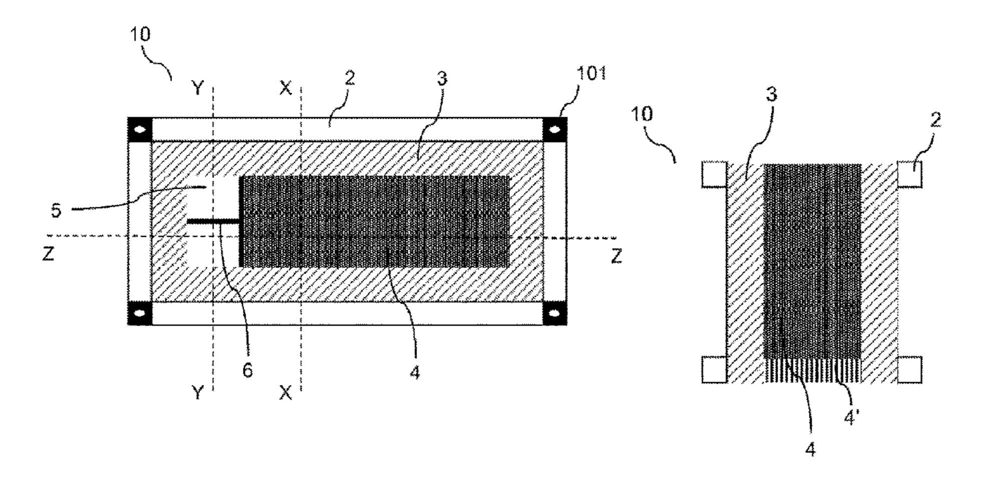
that permits the exchange of mass and/or of heat, the body being parallelepipedal in shape and filling at least part of the chamber, the chamber having an opening on the upper face and/or an opening on the lower face to allow fluid to be transferred to the body from outside the element and/or from the body to outside the element.
