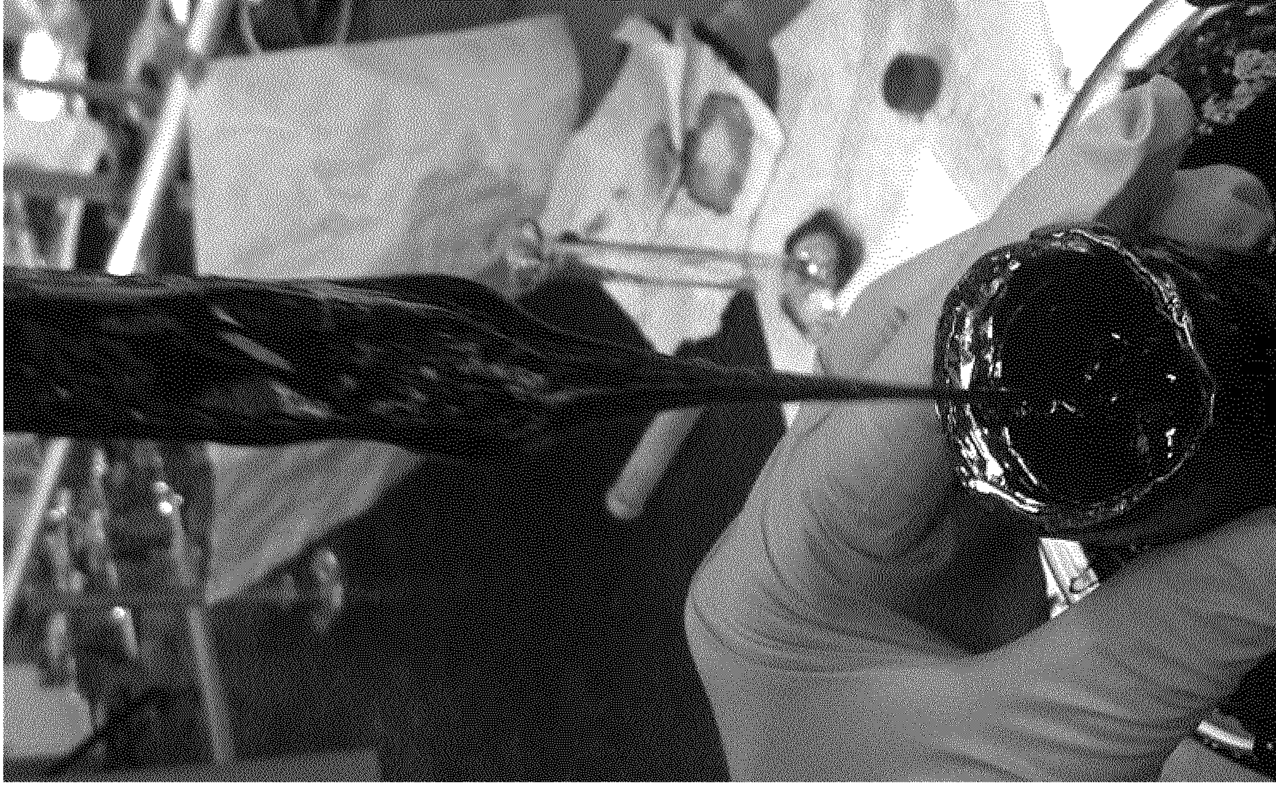
Drainage of heated bitumen from opened pellet
