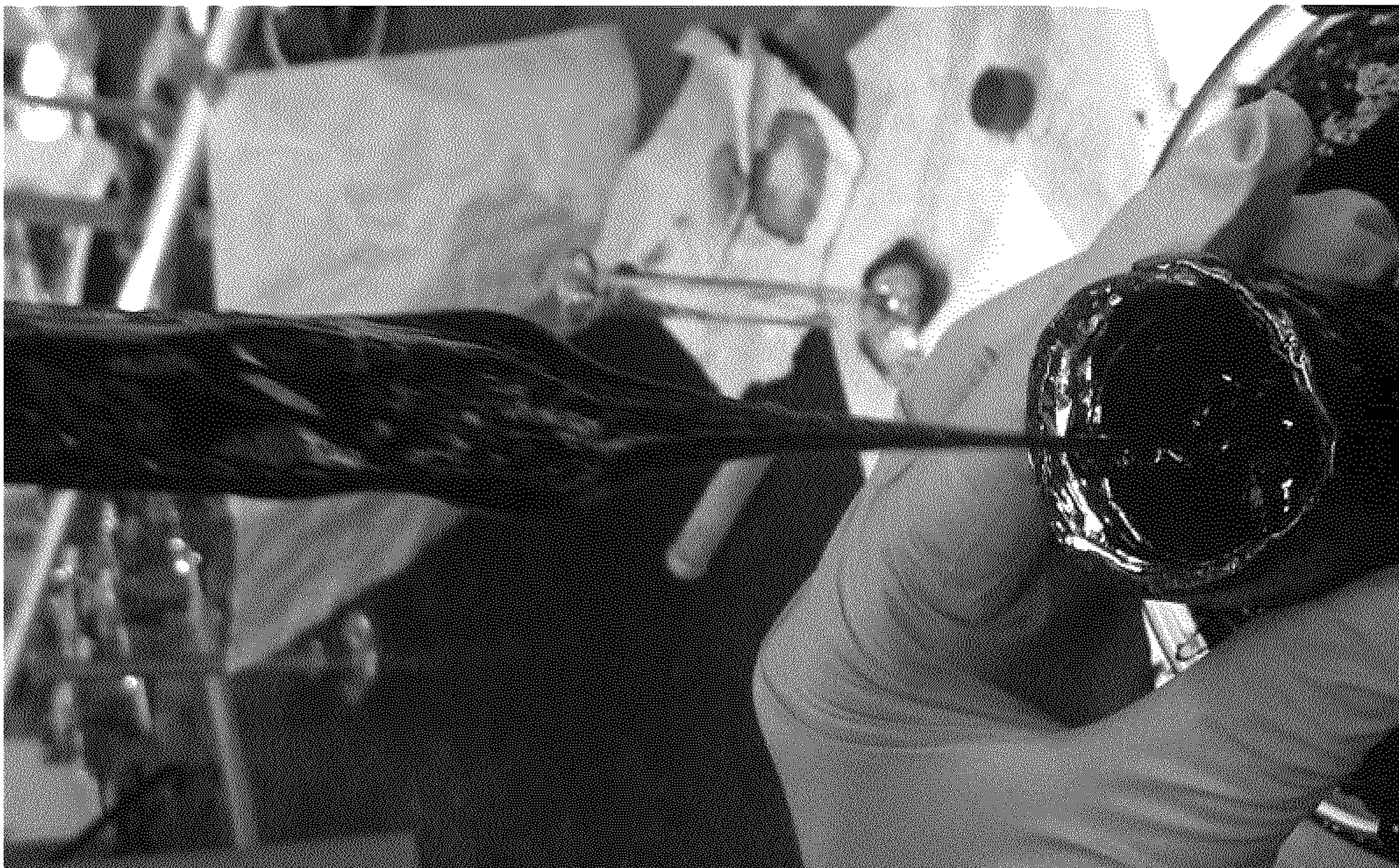
Drainage of heated bitumen from opened pellet
