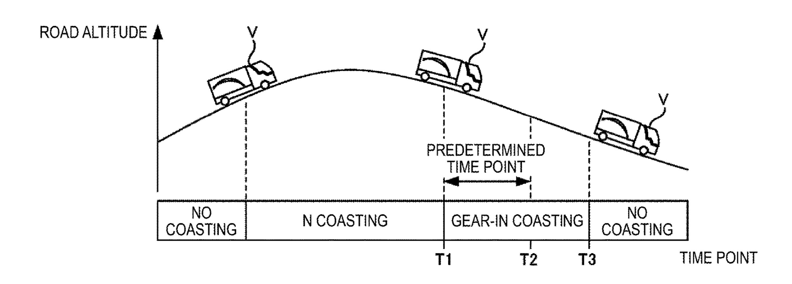
state of the vehicle is the neutral coasting state; and end, the gear-in coasting state when determining that an end condition is satisfied.
