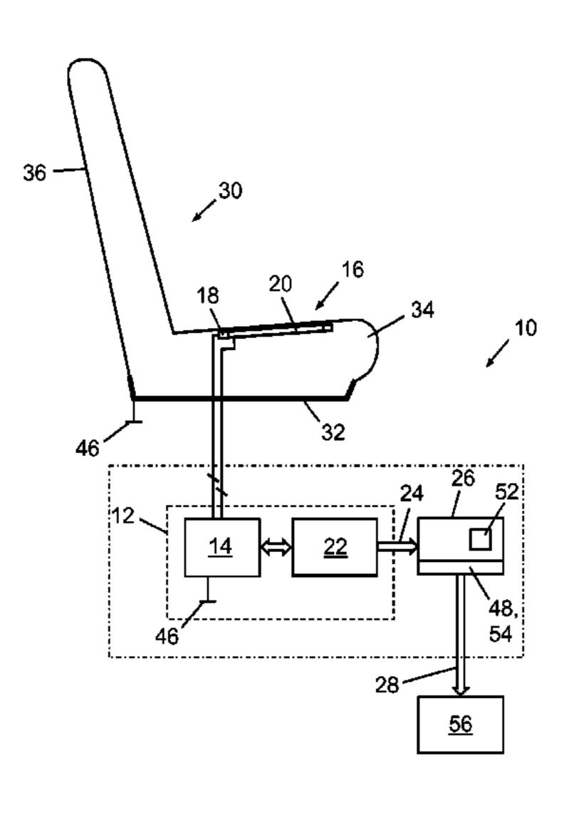
impedance to ground between the two zones the system can get a simplified picture of the impedance distribution on the seating surface. This information can be used to distinguish between grounded structures such as (ISOFIX) child restraint systems and human occupants.
