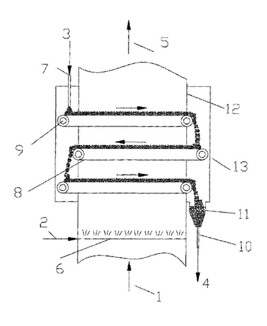
head of a next catalyst support component, making the granular denitration catalyst travel along the catalyst support components reciprocatively.
