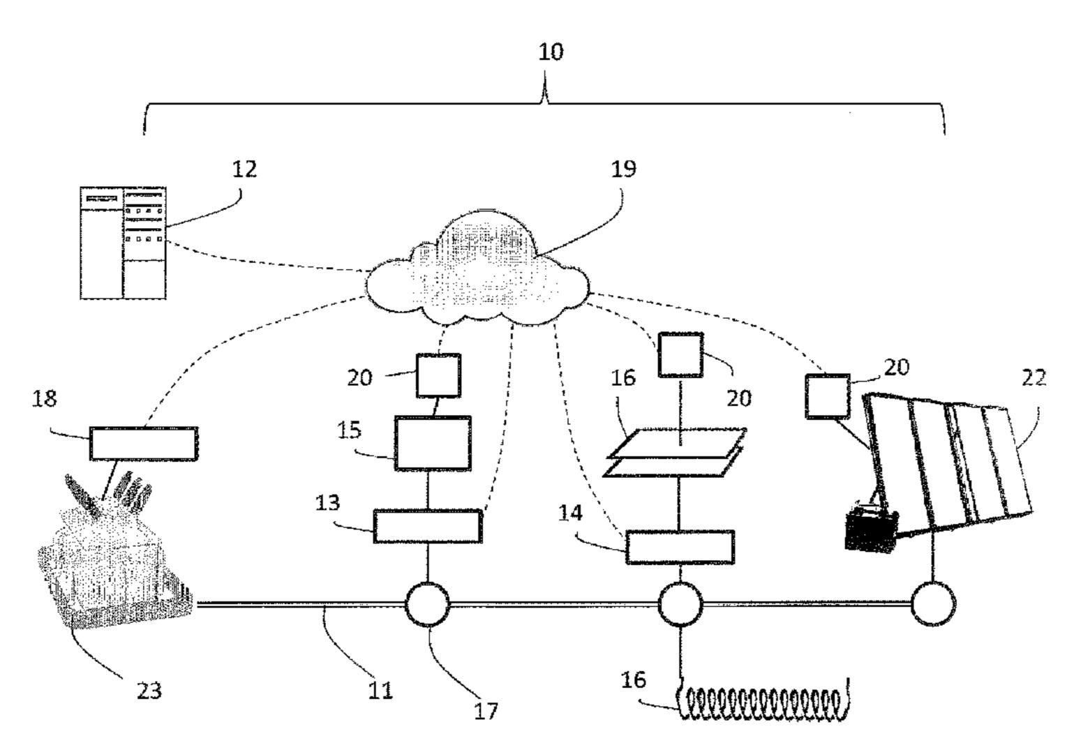
reactive power is injected at the upstream and downstream nodes that consumes all the reactive power in the feeder segment; and adjusting operation of the at least one controllable reactive power resource so that the actual voltage magnitude at the downstream node moves towards a target voltage magnitude of the target voltage phasor.
