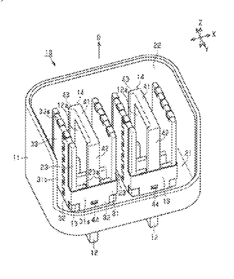
protection caps fixed to the shield members and front end parts of the terminals covered by the front covering portions.
