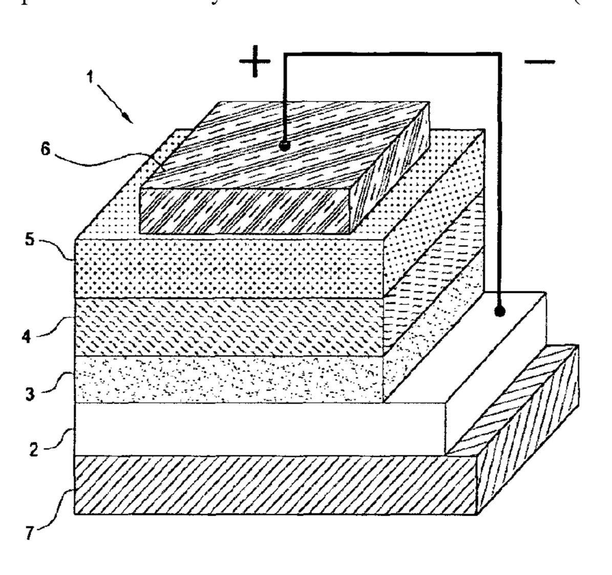
advantageously used in the construction of a polymer photovoltaic cell (or solar cell) with an inverted structure.
