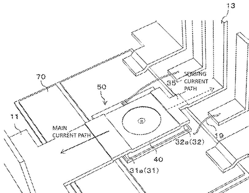
among a sensing current path does not overlap a main current path flowing through the second main terminal 12, the electronic element 95 and the first main terminal 11.
