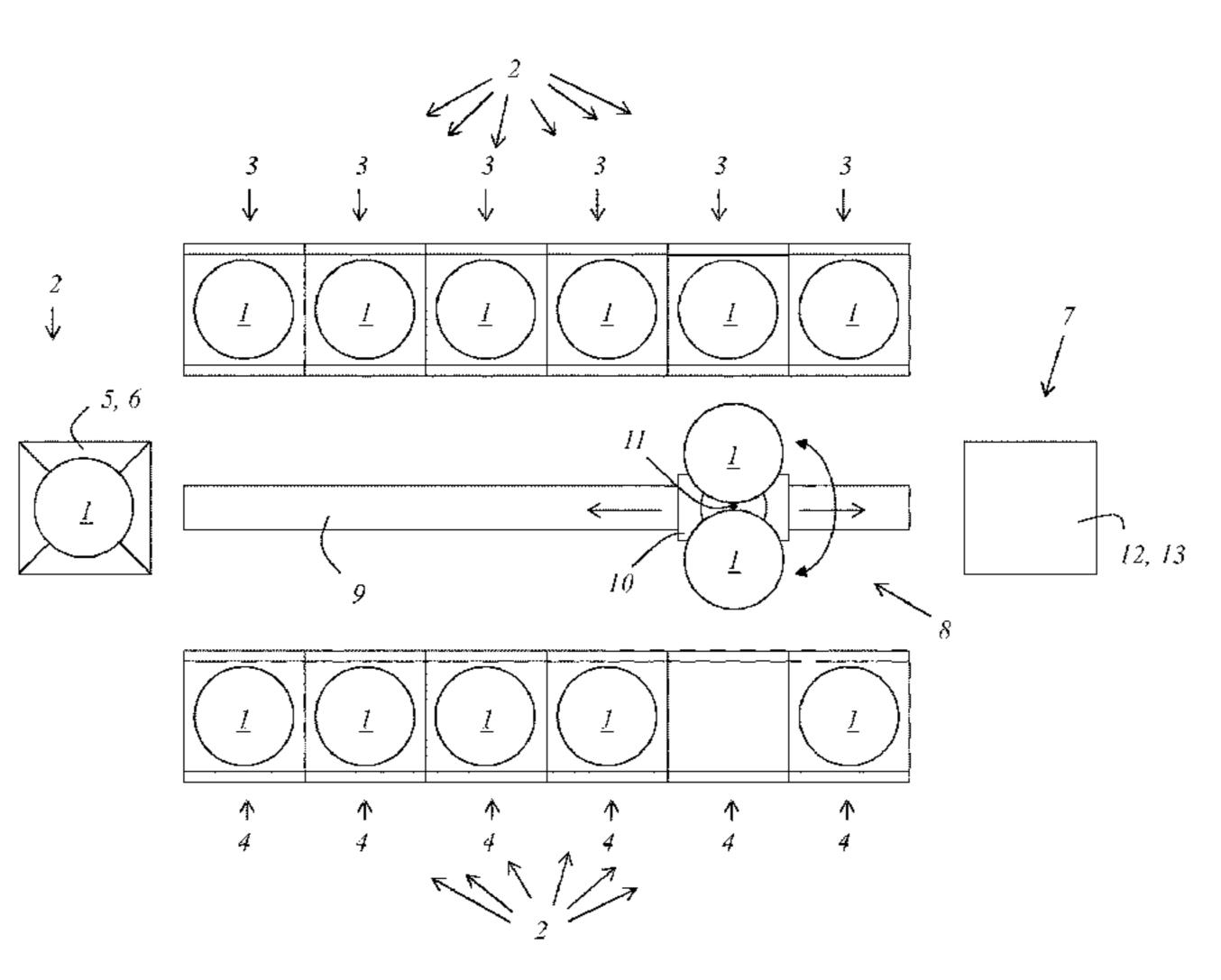
manner, and wherein the spherical receptacle member conjointly with the content thereof and without the rotary drive is in each case retrieved from the processing device which has just terminated a processing step, said spherical receptacle member thereafter being fed to a processing device that is immediately vacant for the respective next processing step.
